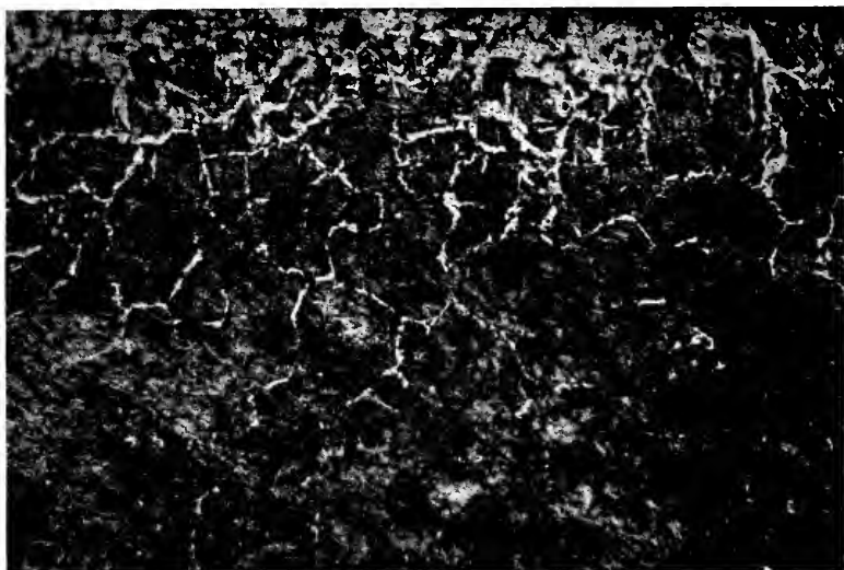
FIG. I.—SHOWING TYPICAL DECARBURIZATION AT SURFACE X100 RAIL No. 7
