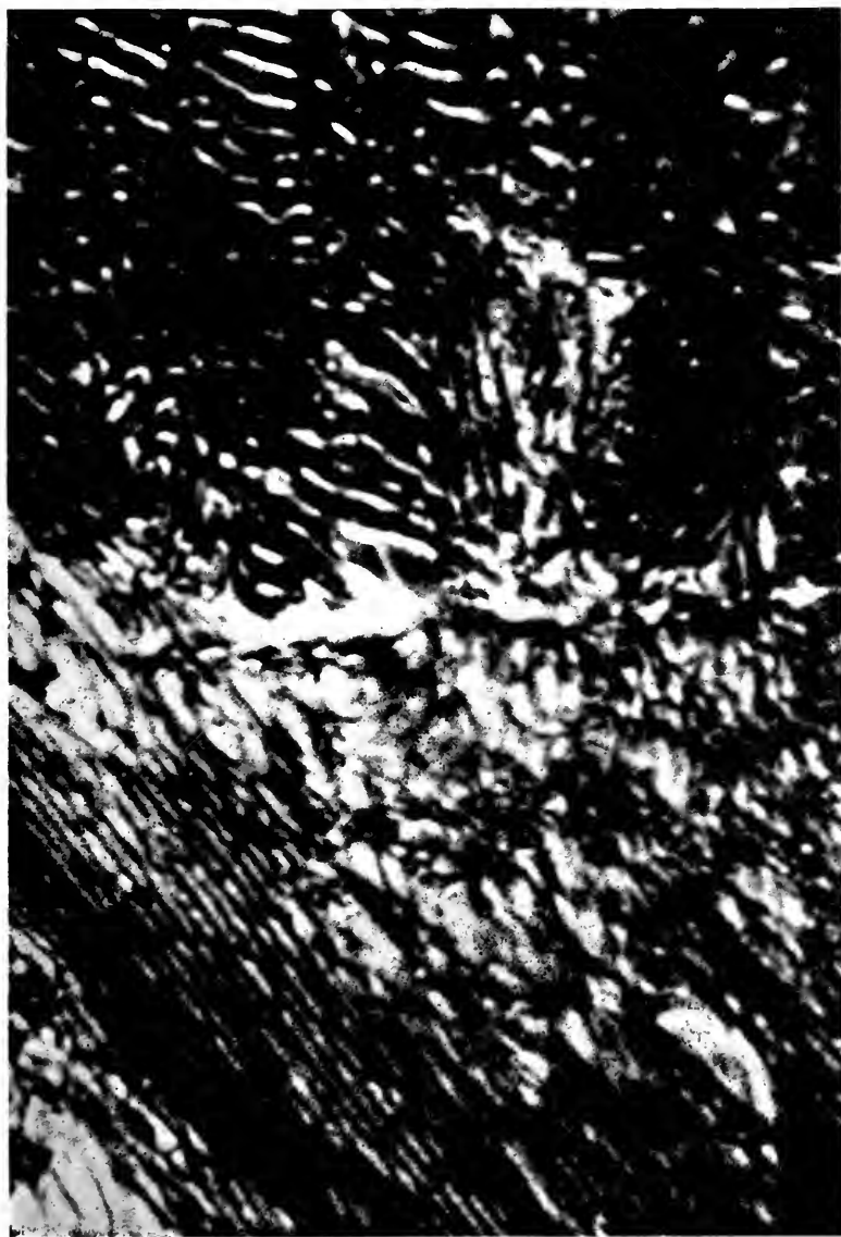
FIG. 15.—RAIL NO. 3 \times 5000. \phi FOR FINE GRAIN = 29^\circ . FOR COARSE GRAIN \phi = 68^\circ .
