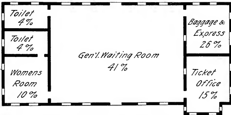
FIG. 1. DIVISION OF FLOOR AREA RECOMMENDED FOR PASSENGER STATIONS WITH ONE GENERAL WAITING ROOM.
