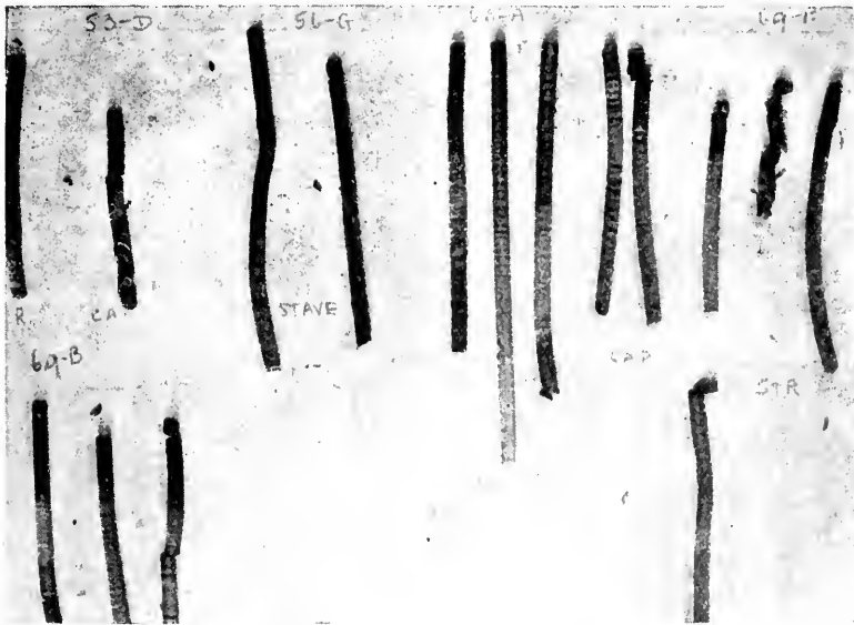
Picture 120. Increment borings from Southern Pacific Bridges 53-D, constructed 1901; 56-G (wood stave culvert) constructed 1900; 60-A, constructed 1900, and 69-B, constructed 1900, indicating penetration of creosote in Douglas fir timber. Also sound condition of timber after 27 and 28 years in service. Photographed August 6, 1928.
