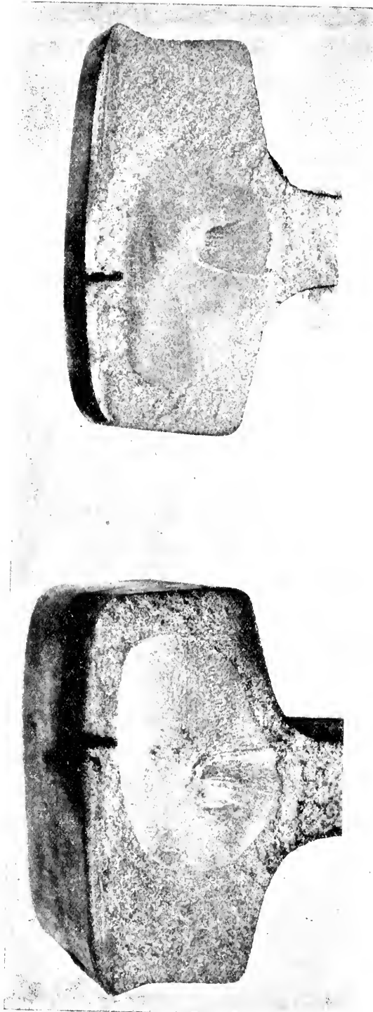
FIG. 1. SHOWING DRILLED FISSURE
