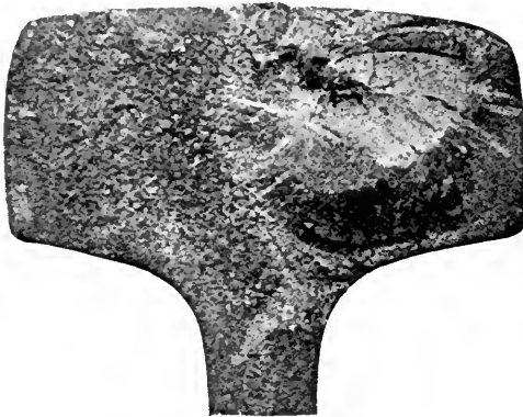
FIG. 6—Specimen L-366-B. 5\frac{1}{8} -inch 80-lb. section. L. I. & S. Co., South Works. Bessemer steel. Heat No. 3718. Rail letter—unknown. Rolled 1901. Failed May 14, 1914. Nucleus of the interior transverse fissure. Cavities.
