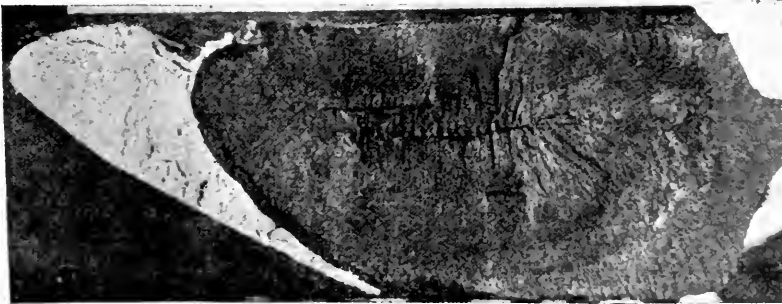
FIG. 1—Showing Horizontal Fissure—Looking Down on Top of Head.
