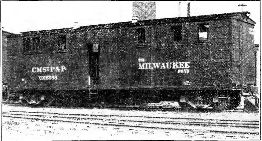
FIG. 4—VIEW SHOWING VENTILATORS AND TANKS.
