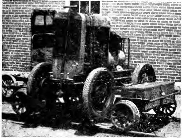
Fig. 6. — Combination Pneumatic Tired Unit Set on Underslung Push Car.
