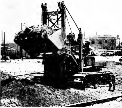
Front-End Loader—Cable Operated \frac{3}{4} Cu. Yd. Bucket Mounted on 40-Hp. Crawler Tractor.
