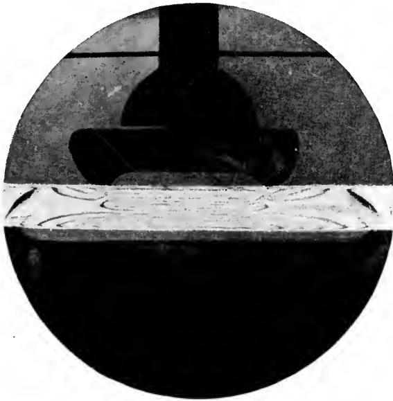
Fig. 1.—Rectangular Bar Under Uniform Bending Moment Through Center Portion.
