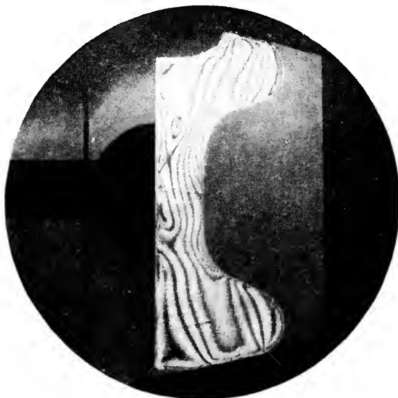
Fig. 4.—Wedge Similar to Fig. 3. Top Fishing Surface \frac{1}{2} in. in Length. Inner Contact Points Symmetrically Located. No Cocking, But Slight Stress Concentration at Top.
