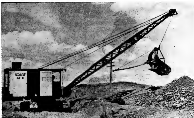
Crawler-Mounted Dragline— 1\frac{1}{4} -Cu. Yd. Bucket.
