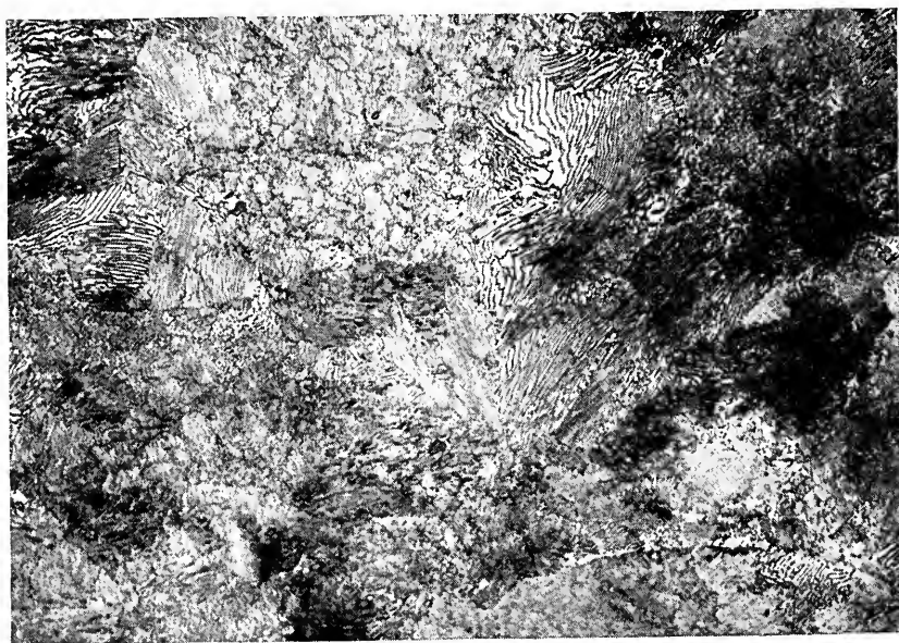
Fig. 14.—This Rail Did Not Shell Although Laid at the Same Time and Adjacent to the Rail Shown in Fig. 15. Note the absence of free ferrite. Picral etch X 500.
