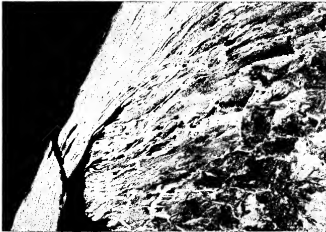
Fig. 12.—An Example of the Flowed Lip of Metal which Forms on the Gage Side of Rail Heads. Note that on the underneath side of the lip a very small crack is evident. Picral etch X 100.
