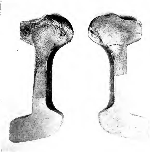
Fig. 2.—Fractures of 132 K-42 Headfree Bars, Bar 133 N and Bar 141 S. Origins of fatigue cracks are indicated by the lines on the curved underside of the head of these bars.
