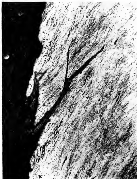
Fig. 10.—Specimen Cut from the Gage Corner of a Rail Head. The oxide-filled crack which is apparent was located on the gage side of the rail. Picral etch X 187.
