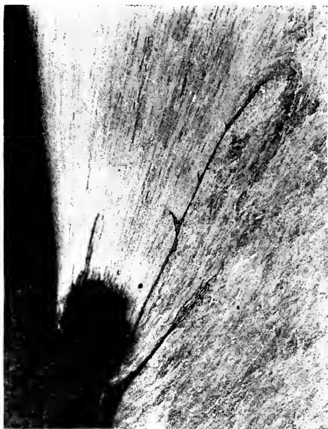
Fig. 9.—Specimen Cut from the Gage Corner of a Rail Head. Note fine cracks filled with oxide that have originated at a position which corresponds to the lowest point of contact between the wheels and rail. Well-developed shelled spots were found at other locations in this rail. Picral etch X 75.
