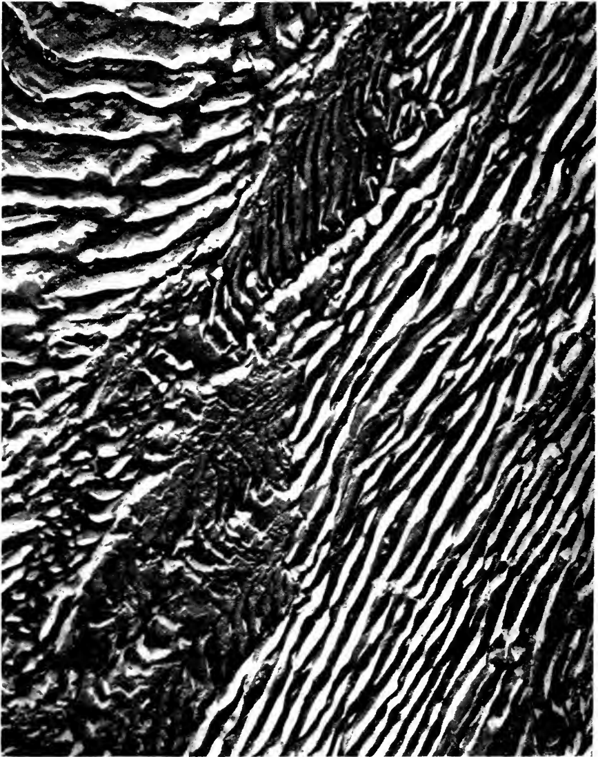
Fig. 11. Electron photomicrograph rail 1137. Magnification 20000 \times . etched in 1-percent nital.
