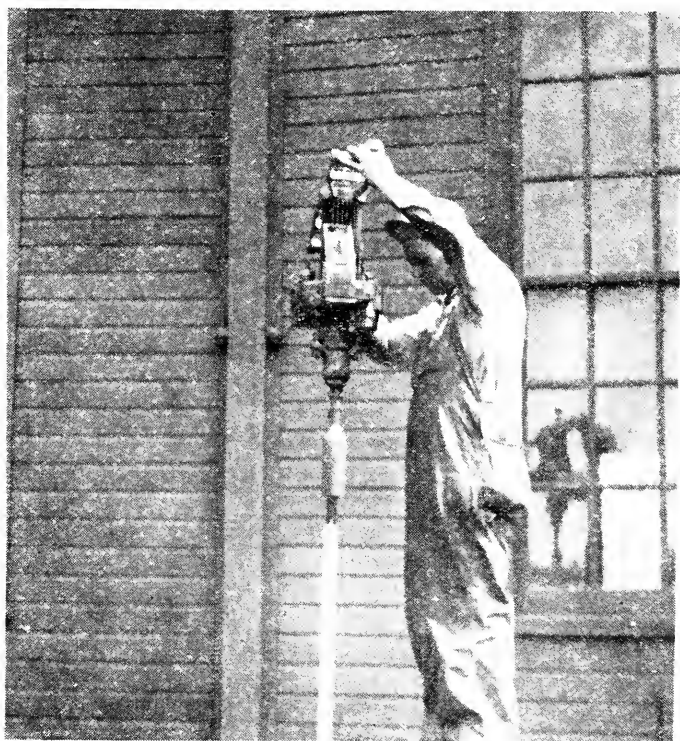
Fig. 4. Unit tamper fitted for driving steel fence posts.
