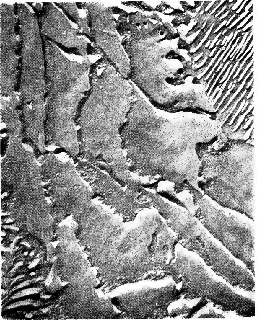
Fig. 8. Electron photomicrograph rail 1123. Magnification 20000 \times , etched in 1-percent nital.
