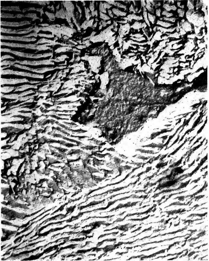
Fig. 9. Electron photomicrograph rail 1124. Magnification 20000 \times . etched in 1-percent nital.
