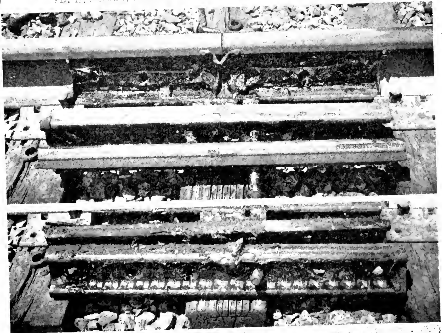
FIG. 14. Section 2, Filled with Petrojatam (Dark) and Plastic End Plugs.
