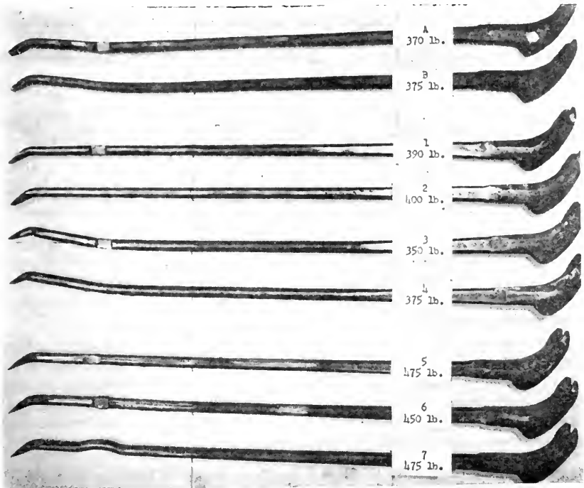
Fig. 9 - Shape of Claw Bars After Bend Tests.
