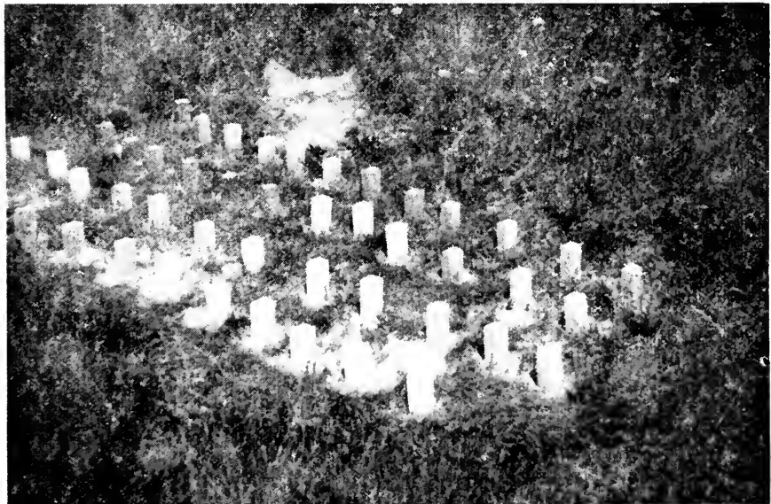
Illustration 6—Field weathering test on 3-in by 4-in by 16-in coated specimens half buried in the ground in an upright position.
