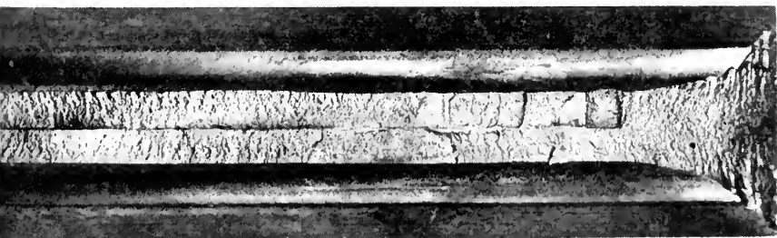
Fig. 6—Pipe in web of an "A" rail which caused failure.
