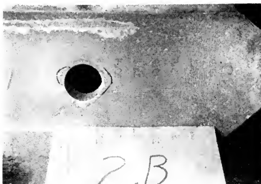
Picture 7. Stress coat pattern around bolt hole of rail end of joint 2S, B side. Pattern outlined with black line due to bolt tension only. Remainder due to tension on entire joint.
