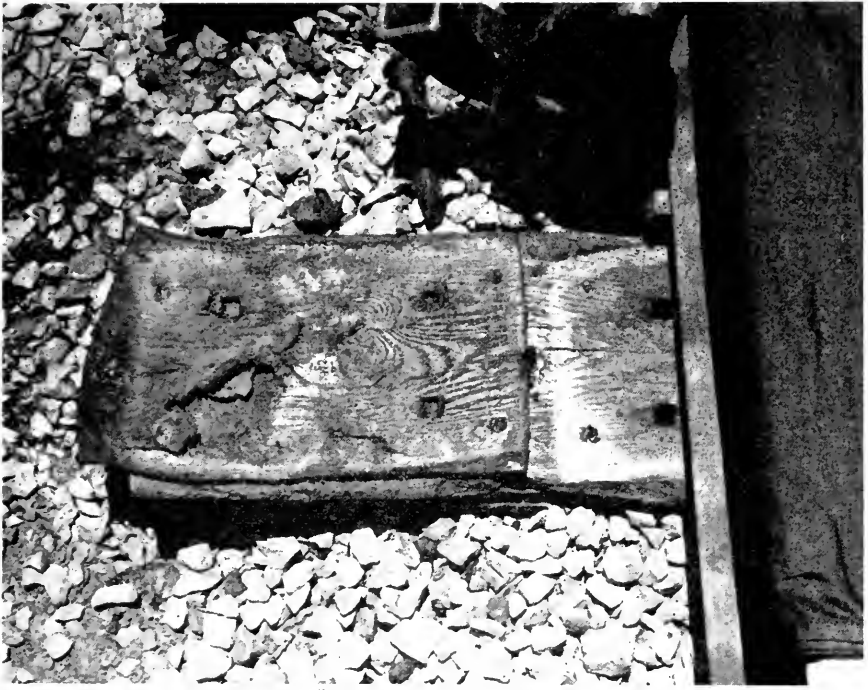
Fig. 11. Section 28, Wool felt Pad (Uncoated), after 33-months' service in the Inner Rail of Long A-cog, 30 min. Curve.
