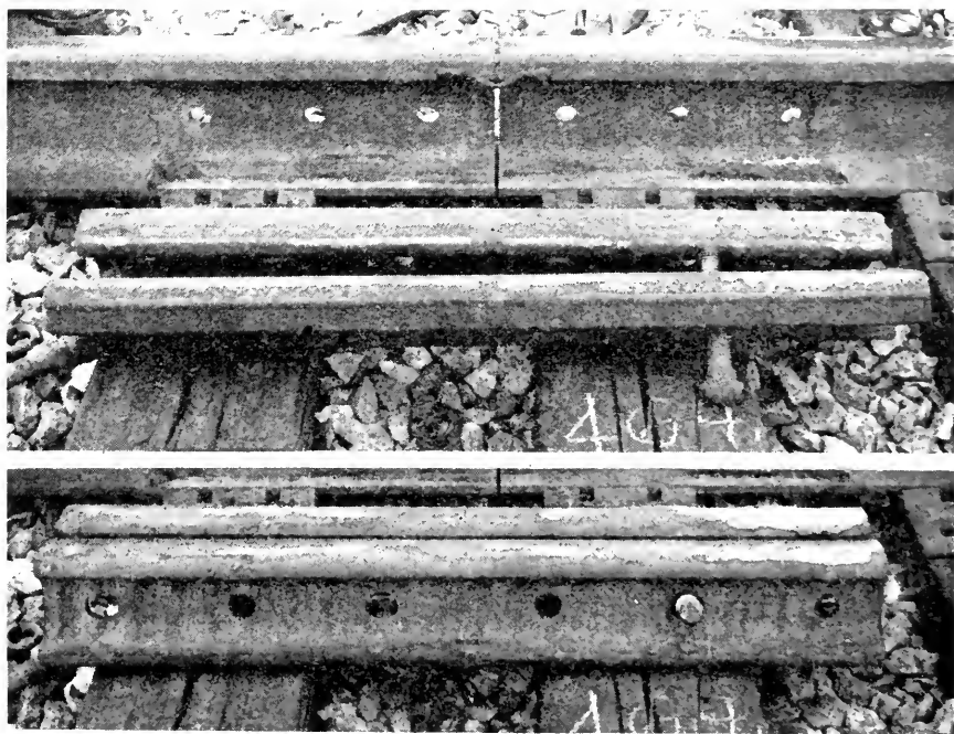
Fig. 8. South Portion of Section 3, Dixon's 1921 Quick Drying Lubricant (Brush coat on rail only).
