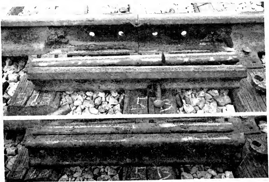
Fig. 10. South Portion of Section 4, No-Cx-Id "A" Special (Brush coat on rail only with No-Cx-Id End Plugs).
