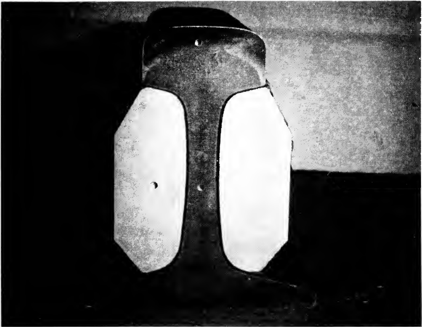
Fig. 1—Full-contact adhesive bonded bars applied to a 132-lb rail section. It can be seen that both bars contact the rail web from the head to the base fillets.
