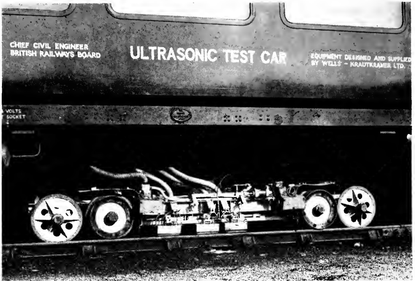
Photograph 5—Ultrasonic rail flaw detection car.
