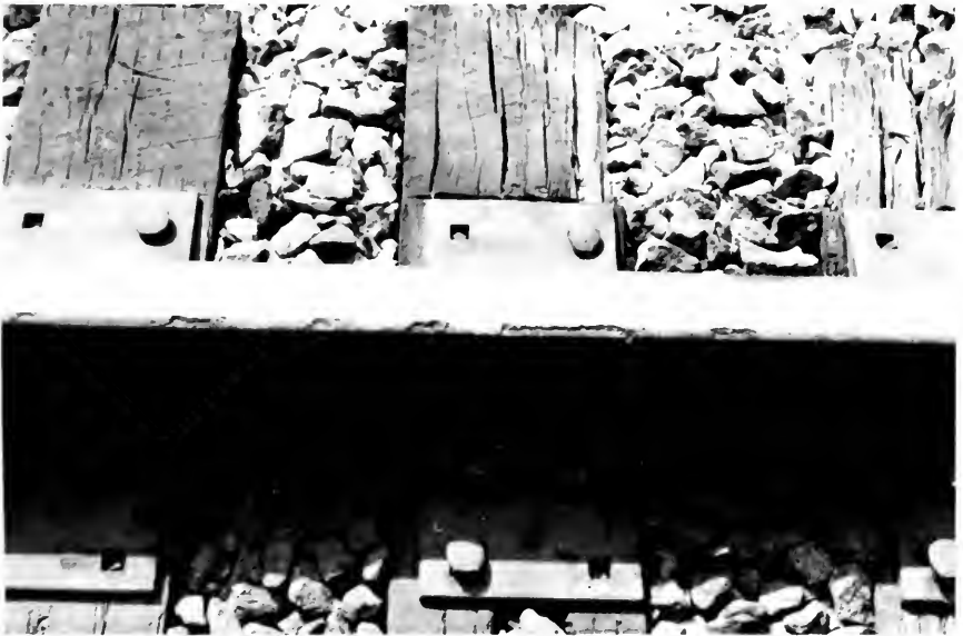
Figure 16. Gage Corner Spalling of a Head Hardened Rail in Well Lubricated Track (Courtesy of A. Merritt, Seaboard System).
