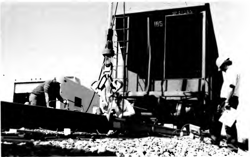
FIGURE 7. RAIL LONGITUDINAL FORCE MEASUREMENT CONCEPT BASED ON RAIL BENDING RESPONSE
