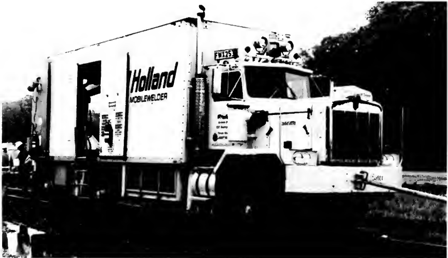
Figure 3. Holland mobile welder at Brandywine, MD.
