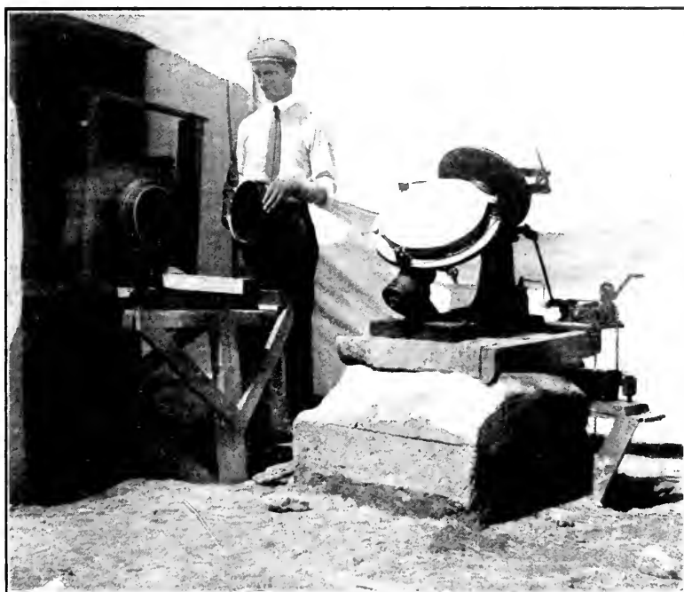
Fig. III. The coelostat and nine-inch lens of the sixty-foot camera.
