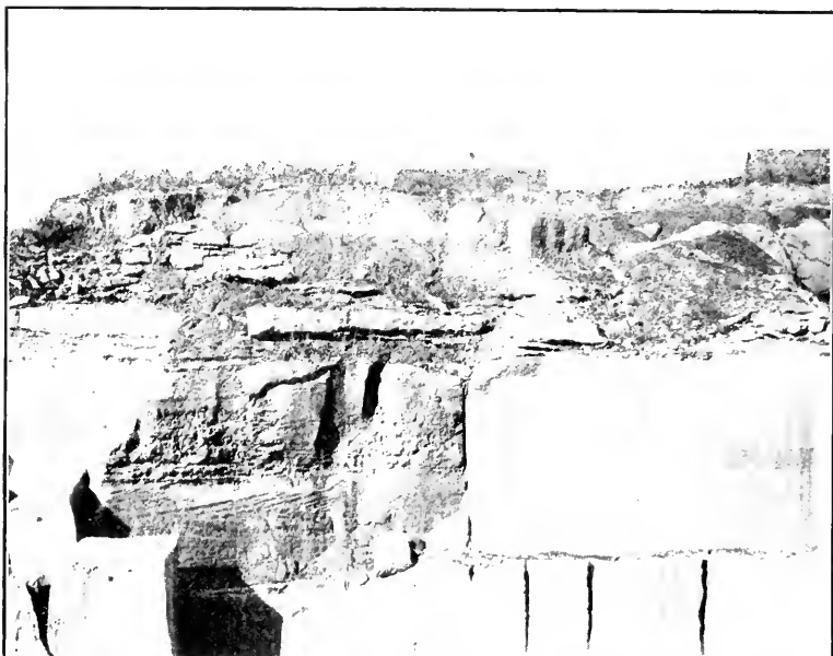
No. 1. Hunter Quarry, Bloomington, Ind., showing fresh quarry face to right and weathered joint face to left. Salem limestone.
