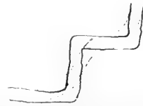
Fig. 4. The solid lines show the original cave and the dotted lines the course the stream will seek to pursue.
