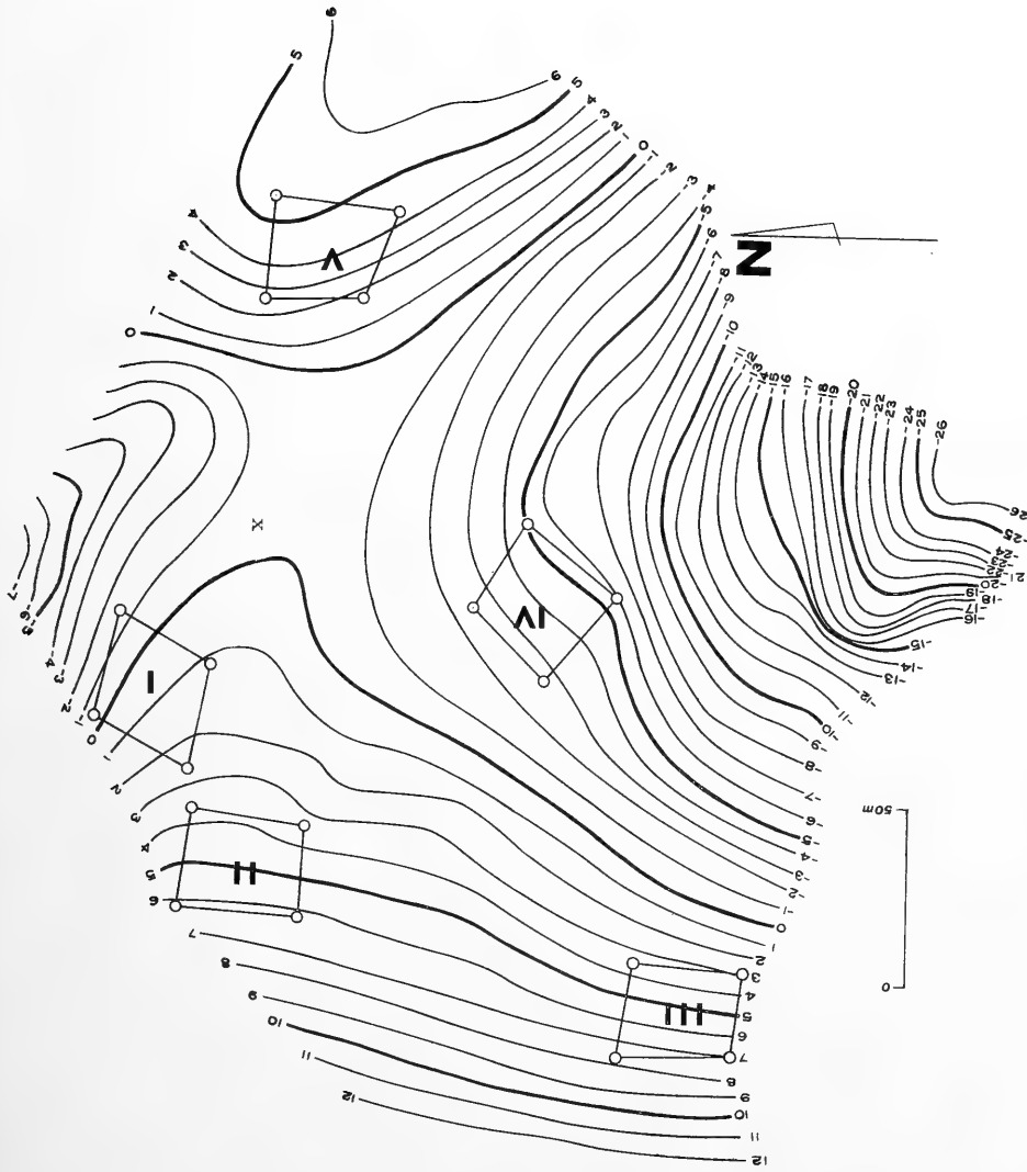
Fig. 1. Topographic map of the area studied at Mourwaring Point showing the position of Grids in relation to contours. Survey datum position (x) map reference 8/431/597. Height contours relative to datum position in metres.
