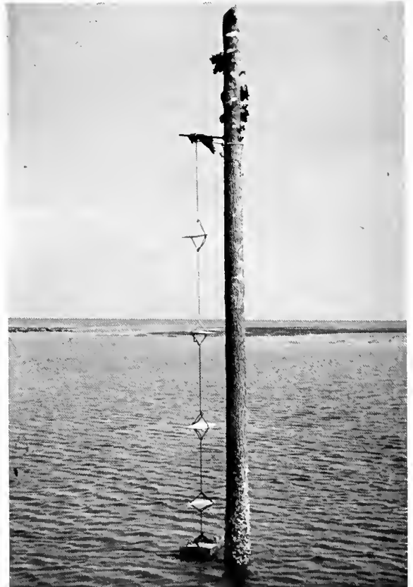
FIG. 3. Intertidal field transect station at low tide showing panel placement. The halter line is secured at the bottom by a solid cement block and at the top by a metal rod extending perpendicularly from the stake.
