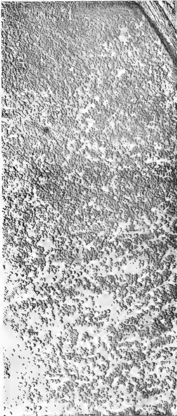
BLOCK OF BANCA TIN WITH TINPLAGUE. Inoculated with grey tin; in solution of pink salt. 27 Sept. — 13 Oct. 1899. Temp. —5° C. Enlargement 1½ lin.
