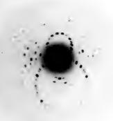
Fig. 1. Turmaline. Plate parallel to (0110).
