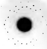
Fig. 14. Quarz. Plate parallel to (1210). (Abnormal Pattern). PLATE IV.
