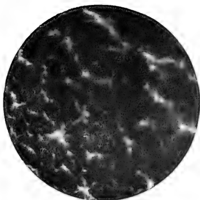
Fig. 4. Molybdenum (heated in vacuo). v = 800 \times .
