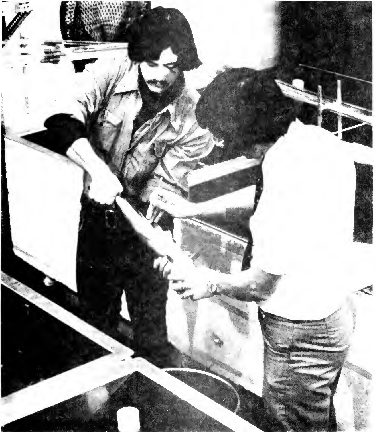
Figure 2. Laboratory evaluation of chronic effects of contaminants on fish in a flow through diluter system.
