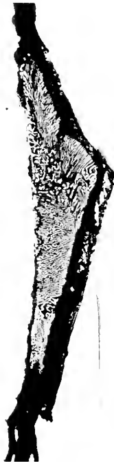
FIG. 2. A plessite field with a pearlitic structure of kamacite and taenite lamellae, almost surrounded by hydroxide. At this magnification it resembles similar areas of pearlitic structure in a number of other irons (e. g., Leeds, Seelasgen, Youdegin) in which the white lamellae are kamacite and the gray are taenite. Pical 30 seconds; \times about 40.
