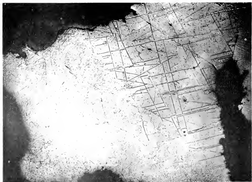
FIG. 2. An area at the edge of the slice showing, at lower left, a zone of alteration in which the normal structure has been replaced by a secondary granulation. The dark area at lower right is probably hydrosidite; that at upper left is silicate. Pical 120 seconds; \times about 30.
