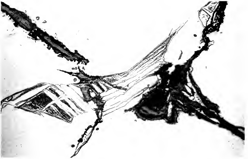
FIG. 1.--An irregular plessite field containing lamellae of taenite (gray) and small areas of incompletely transformed gamma-alpha aggregate. Small schreibersite bodies surrounded by hydroxide. Pical 85 seconds; \times about 35.
