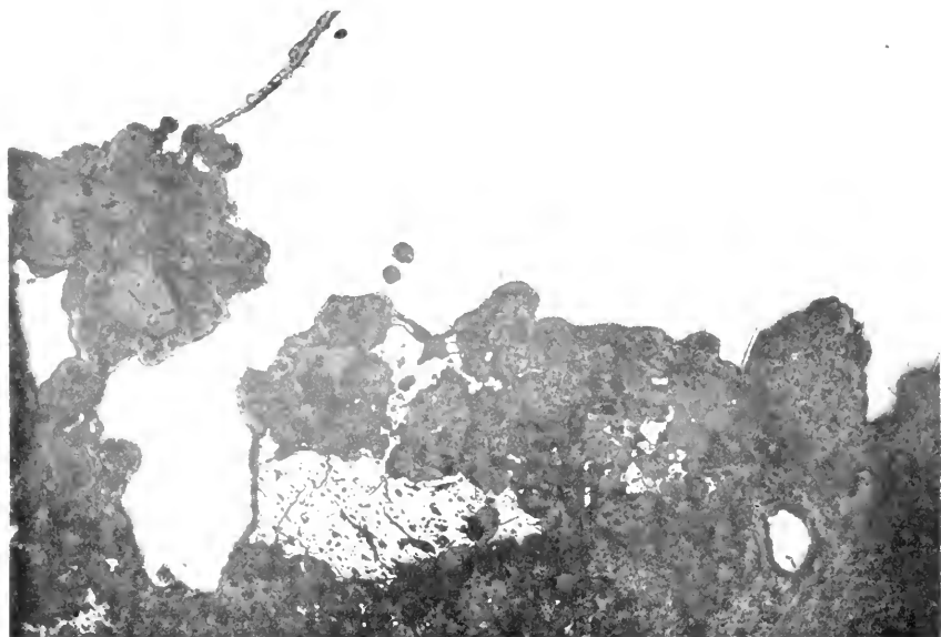
FIG. 1.—Irregular edge of an inclusion. The silicate at one point extends in a streamer from the mass. Three small isolated particles of silicate in kamacite. Pical 30 seconds; \times about 45.
