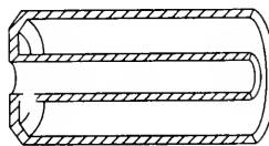
An integral center tube can be formed so that assembly and machining are not needed.
