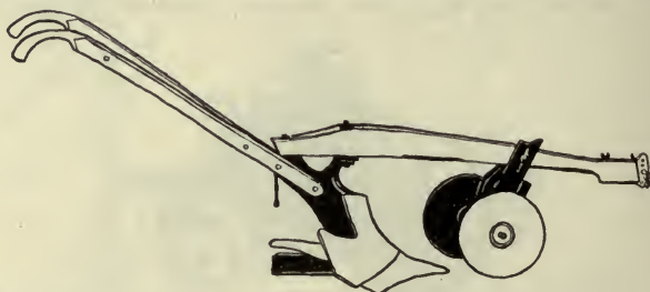
FIG. 120.—Special plow, fitted with two rolling coulters for digging sweet potatoes.
