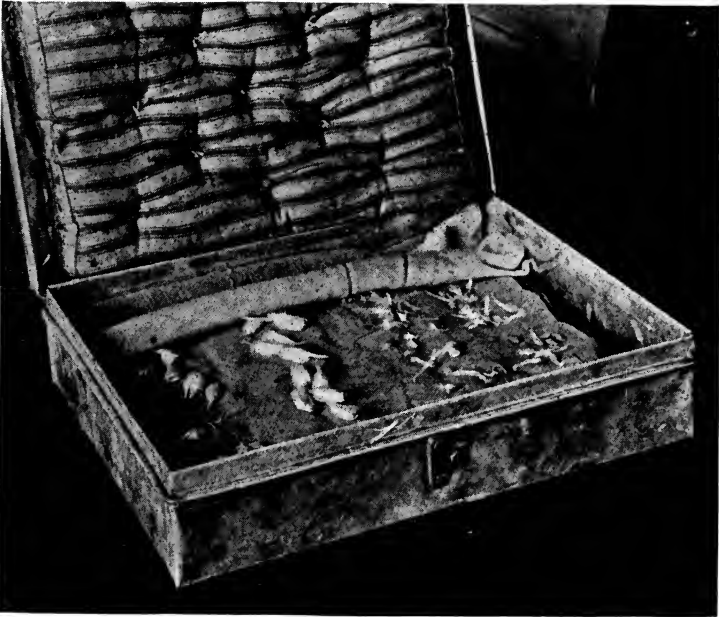
FIG. 7.—A box germinator. A tin box with two sawdust pads. Can be carried about.
