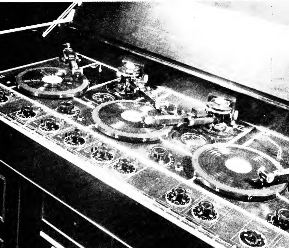
Figure 33. Turntables constructed as portable units.
