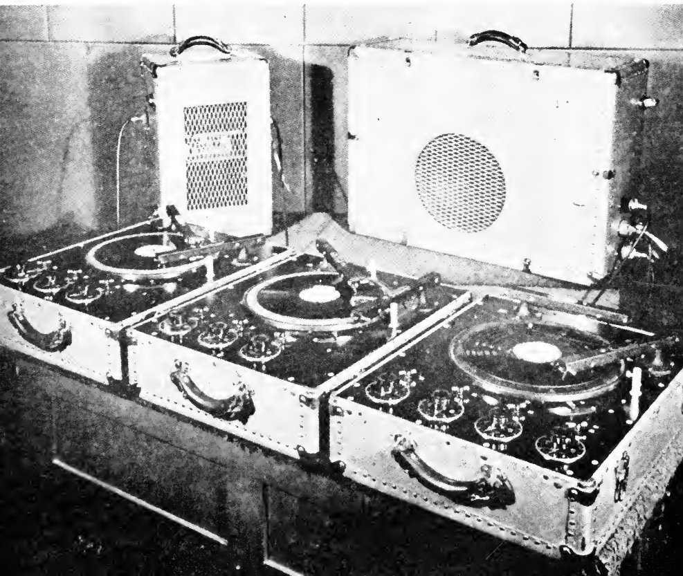
Figure 32. Close-up of the triple turntable showing spotting arms.
