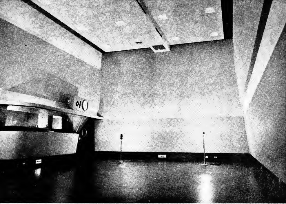
Figure 7. Live-end dead-end studio with slanting walls.
