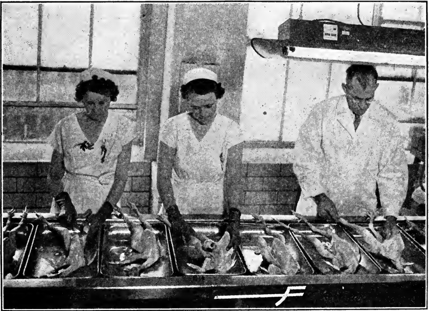
FIG. 112.—Clean-up and inspection stations at the end of a disassembly line. (Courtesy of Jerpe Commission Company.)
