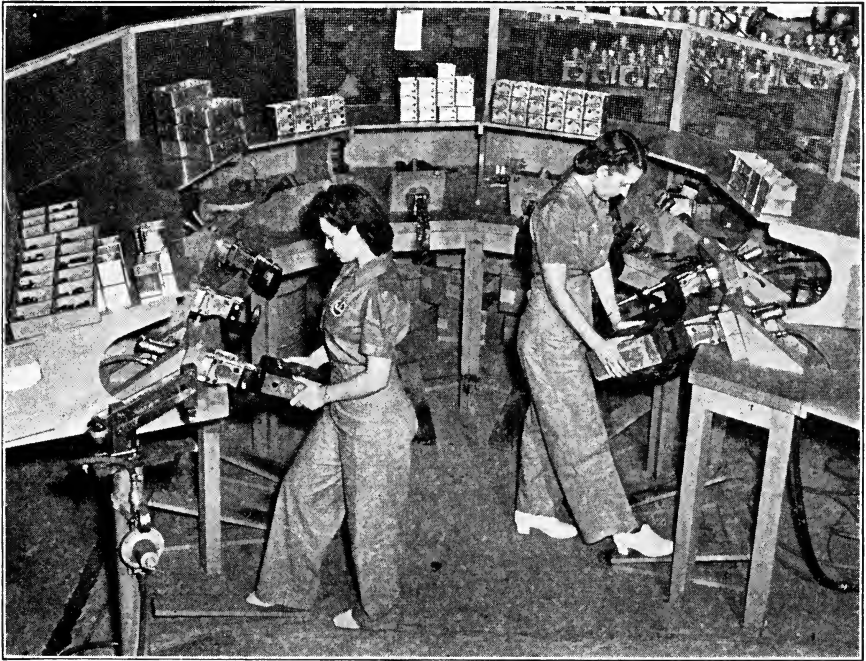
Fig. 111.—Both operators and work move on this line. Each girl carries the complete unit through all operations. ( From American Machinist. )
