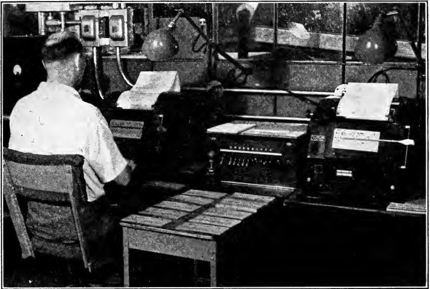
FIG. 86.—At the control booth in a truck-assembly plant the operator is seen sorting the order cards and dispatching, via teletypewriter, the assembly building sequence to various stations along the final and subassembly lines. (Courtesy of Dodge Division, Chrysler Corporation.)
