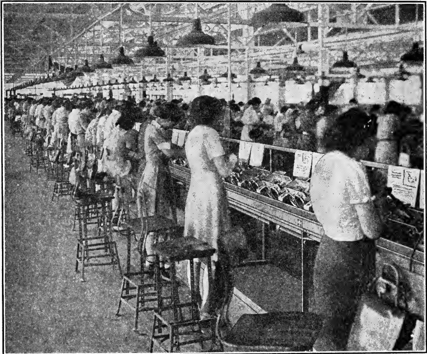
FIG. 28.—On this conveyor are mounted special fixtures to hold the radio chassis in position while the assembly operations are performed. (Courtesy of Logan Company and Radio Corporation of America.)
