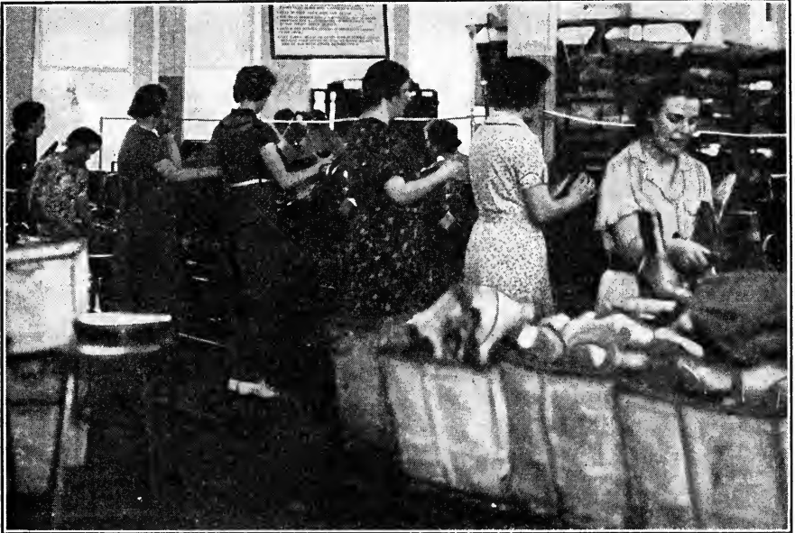
FIG. 101.—This rubber-shoe assembly line is a paced production conveyor with a wage incentive. The speed of the line is as fast as the operators wish it to be set, but any worker can stop the line momentarily by merely pulling the cord above the line in the event of minor delays in her operation. The line may restart automatically after several sec. or may be set to begin again only after one of the operators again pulls the cord. (Courtesy of United States Rubber Company.)
