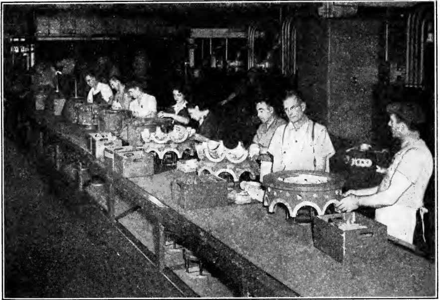
FIG. 20.—This simple belt conveyor line masks out certain areas on these aircraft motor parts before they are painted. Each worker has his specific operations of placing corks, tape, or wood blocks at the points needing protection. ( Courtesy of Ford Motor Company. )
