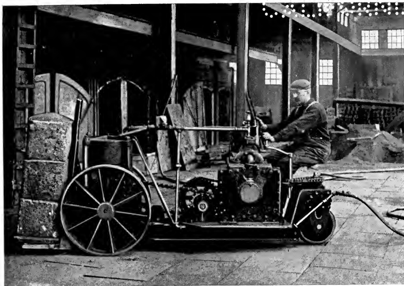
Fig. 28—Pneumatic charging machine which serves the annealing furnaces, charging and discharging the pots
