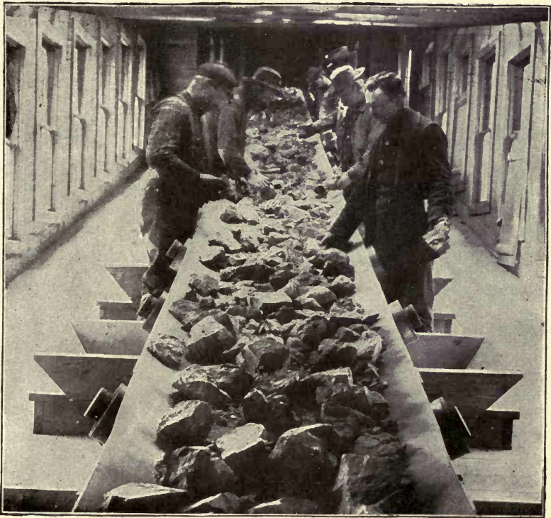
FIGS. 23 AND 24.—ROBINS CONVEYING AND PICKING BELT.
