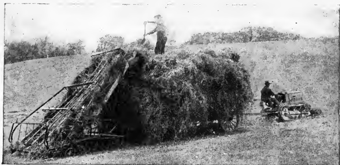
FIG. 243.—A caterpillar tractor drawing a wagon and hay loader. (Cleveland Tractor Co.)
