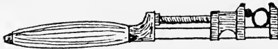
FIG. 241.—A monkey wrench and round file may serve as a pipe wrench.
