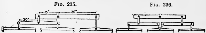
FIG. 235—This three-horse evener is easily constructed by attaching a single-tree and a two-horse evener to a new triple-tree divided as shown. FIG. 236—One of the best forms of a three-horse evener.
