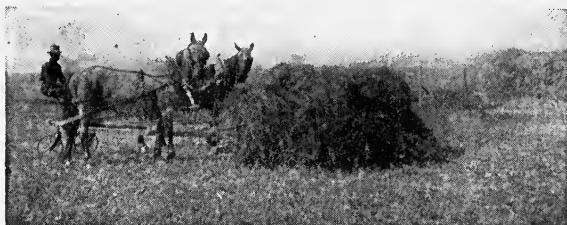
FIG. 57. —Push power sweep rake used in taking hay to a stack in the field. (Plant Industry.)
