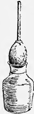
FIG. 6.—Osmosis with an egg over a bottle of water. If egg liquid and the water exchange places through the membrane of the egg, which moves the faster? Why does fluid rise in tube?
