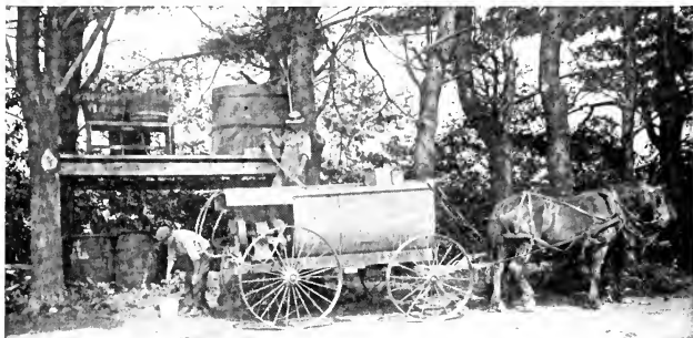
FIG. 82.—A gasolene power outfit. The most efficient power sprayer. The cut also shows an excellent arrangement for filling the tank and mixing the materials.
