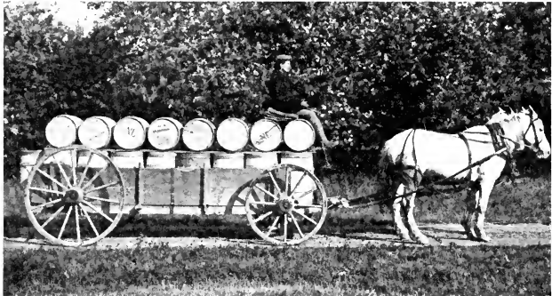
FIG. 118.—A load of apples on the way to market. This is a good type of wagon for hauling barrels. It is low, making it easy to load, and it will carry twenty-five barrels easily.
