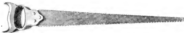
FIG. 59.—The two-edged saw. An abomination that ought to be banished from the orchard.
