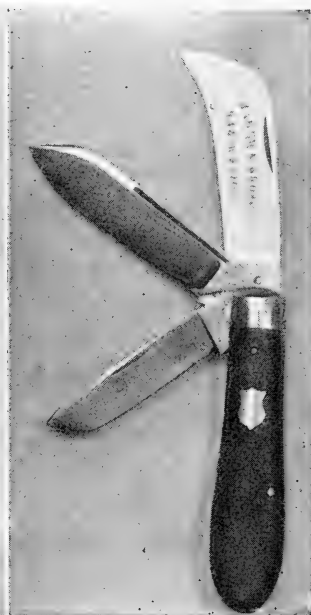
FIG. 64.—A good type of pruning knife. Long hooked blade and large enough for heavy work.
