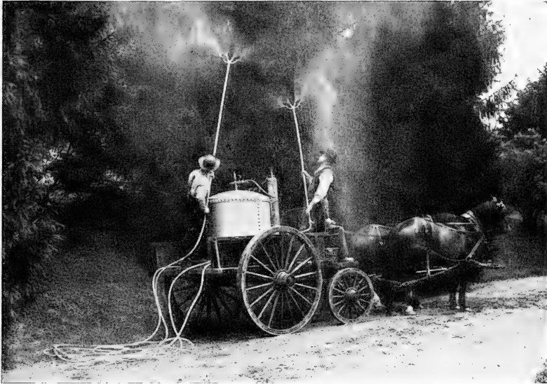
FIG. 81.—Gas power sprayer. An excellent type in some respects, but it is too difficult to clean out the tank.
