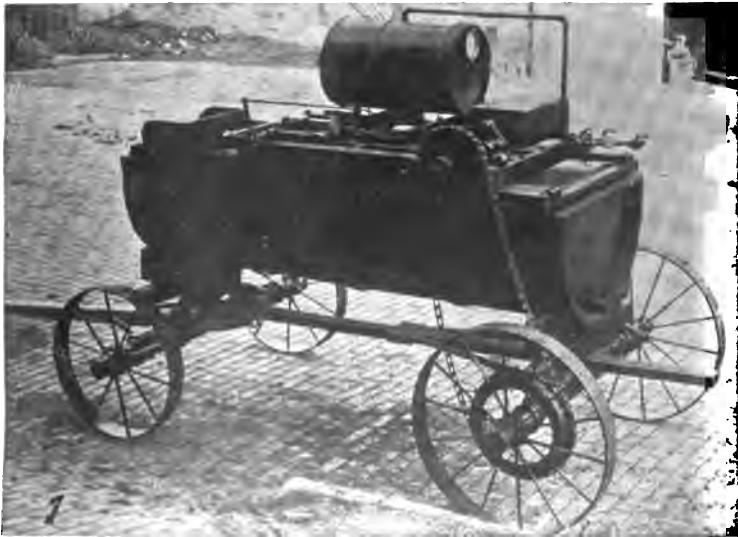
FIG. 299.—Spraying outfit with tank for liquid below, air pressure tank above, and air pump operated by chain gear from hub of truck wheel. (Fights of the Farmer.)
