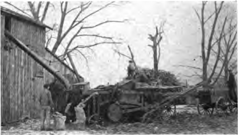
FIG 135.—The corn husker and shredder removes the ears and carries them to the rear where they may be caught in a wagon box. It shreds fodder very fine and blows it into a suitable storage place. Any corn shelled may be caught in bags, as shown. (I. H. Co.)
