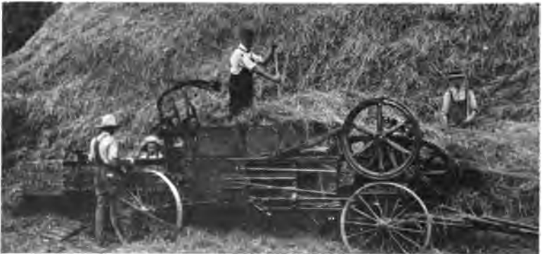
FIG. 111.—Baling straw with engine-driven press. Note the self-feeding arm above. (I. H. Co.)
