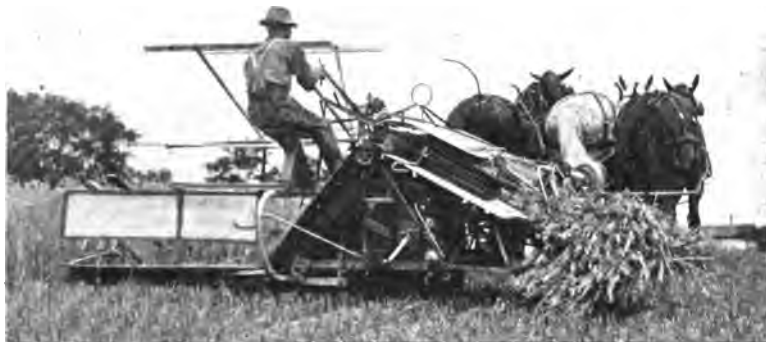
FIG. 151.—Harvesting grain with modern self-binder. (I. H. Co.)
