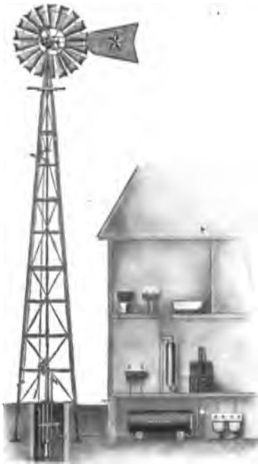
FIG. 310.—Hydro-pneumatic pressure system with tank containing air and water under high pressure. The pressure is maintained with a pump operated by engine, motor, or wind mill. (Flint and Walling Mfg. Co.)
