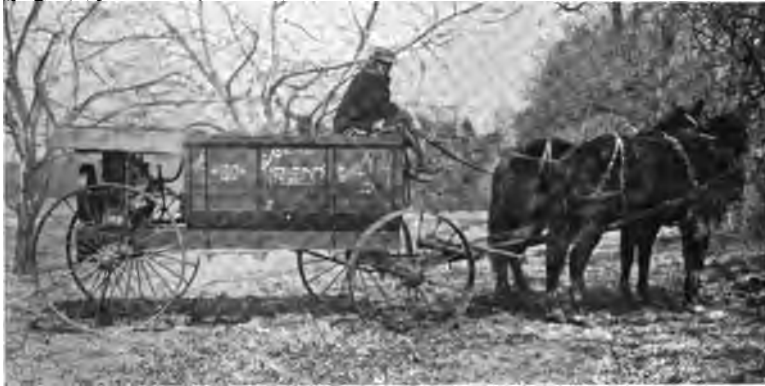
FIG. 298.—Spraying is much less laborious when a gas engine is employed for the work (New Jersey Station.)
