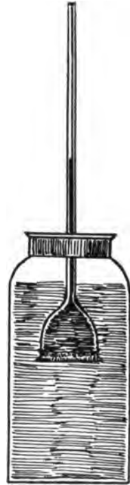
FIG. 5.—Osmosis with a bladder membrane tied on mouth of funnel tube. After the bladder is tied in place, the tube is filled with thick syrup or other strong solution. Water is in the large bottle. As the osmosis takes place the liquid may ascend the tube many feet if it is extended high enough.
