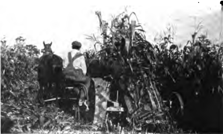
FIG. 137.—This type of corn harvester cuts the crop, ties it in bundles and throws them to one side. (Productive Farm Crops.)
