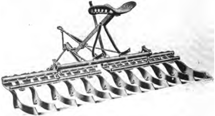
FIG. 67.—The Acme harrow is a good clod crusher. When the soil surface becomes pulverized the moisture is conserved.
