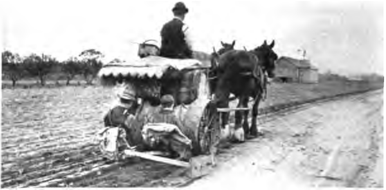
FIG. 255.—Machine at work setting tobacco plants in the open field. The boys behind place the plants in the planting pocket one at a time. The machine opens the furrow, waters the plants, and presses in the soil around them. (U. S. D. A.)
