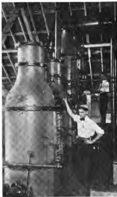
FIG. 211.—Interior of a sugar cane mill, showing the vacuum "pans." The sap is evaporated under pressure much below that of the atmosphere to lower the temperature of boiling. (Louisiana Station.)
