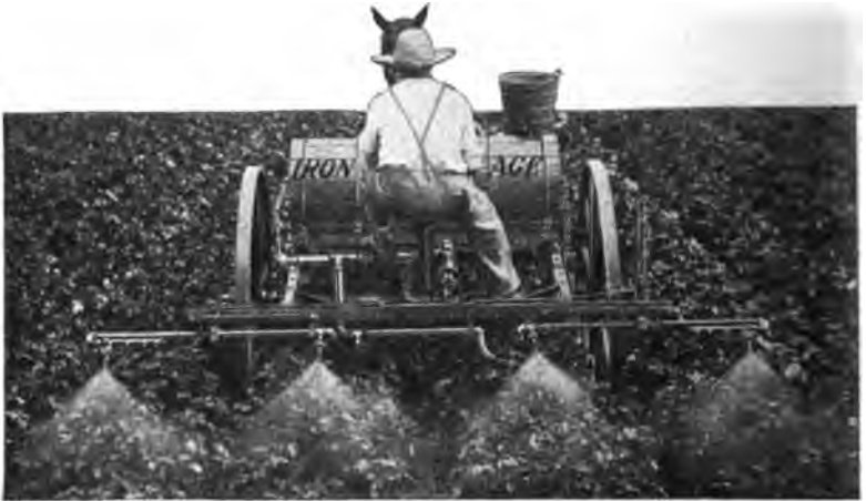
FIG. 295. —This four-row sprayer is operated by chain gear on the axle. It is suitable for spraying potatoes, cabbage, and other truck crops. (Courtesy Osborn Co.)
