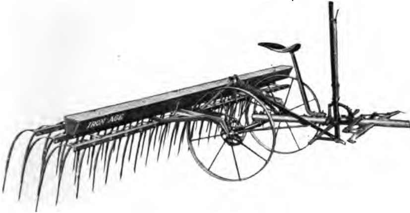
FIG. 68.—The weeder will produce a fine dust mulch and conserve moisture in the soil. (Bateman Mfg. Co.)
