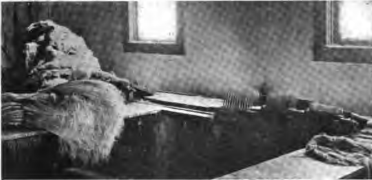
FIG. 199.—Flax hackles. Dressed or hackled flax is prepared by drawing the scutched fibre first over the coarse hackle, then over the finer ones, combing out shives and coarse and tangled fibres. (U. S. D. A.)
