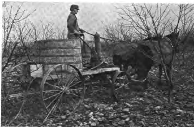
FIG. 293.—A spray pump operated by hand which pumps the liquid from the big tank and delivers it at high pressure through the spray hose. (New Jersey Station.)
