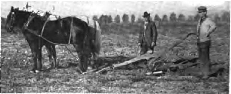
FIG. 165.—This simple potato digger has several tines instead of a moldboard, allowing the soil to fall through but keeping the potatoes on top. (New Jersey Station.)
