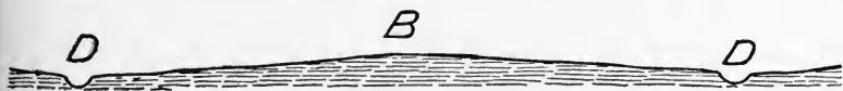
FIG. 47.—Dead furrows as drains. On tight soils, especially on fields having little slope, surface drainage may be had by plowing in narrow “lands” up and down the gentle slopes. The surface water drains from the back furrows to the dead furrows, thence down the dead furrows and off the field. B , back furrow; D , dead furrow. (See Fig. 68.)
