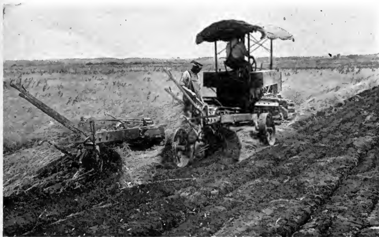
FIG. 194.—Two twenty-four-inch bottom plows turning tough marsh turf. (Wisconsin Station.)
