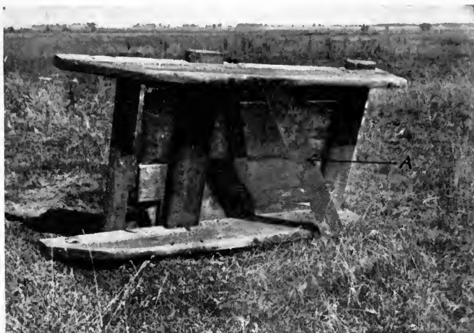
FIG. 197.—A bog cutter. Note the cutting blade (A) extending from runner to runner.
