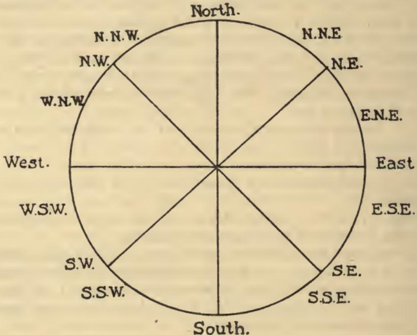
be correctly oriented. An easy way to do this is to have two sticks below the gauge crossed at right angles, one marked on the end with "N" for north. The arms can then be so set that "N" points to the north, as determined either by the sun at midday, the polestar at night, or the compass (remembering that the magnetic north is  $13^{\circ}$  west of the true north).
