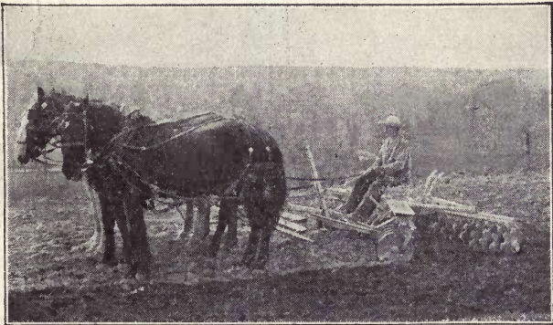
No. 23. Tandem or Double Disk Harrow One man with six horses with this device will do double the work one man and four horses with a single disk. See page 29.
