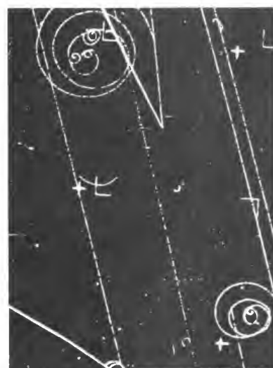
In this bubble-chamber picture, a neutron is produced at the bottom, at the end of the 1.25-cm long track, near the + mark. This neutron in turn causes a reaction near the center of the plate. (Neutral particles do not leave tracks in bubble chambers.)
