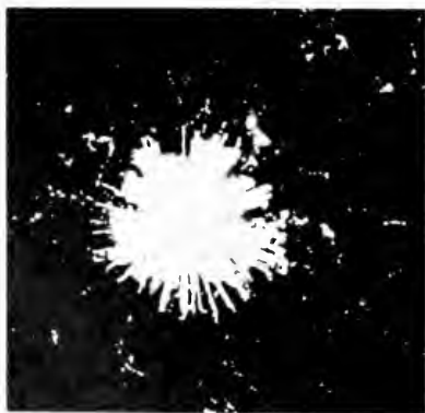
A grain of radioactive dust from the atmosphere caused these \alpha -particle tracks in a photographic emulsion (enlarged 2000 times).
