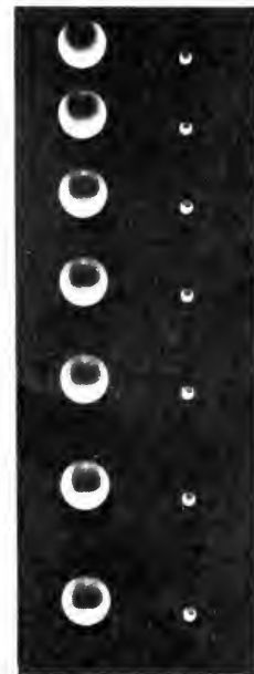
A stroboscopic photograph of two freely falling balls of unequal weight. The picture shows the last part of the total path. The balls had been released simultaneously. The time interval between images is 0.03 sec.
