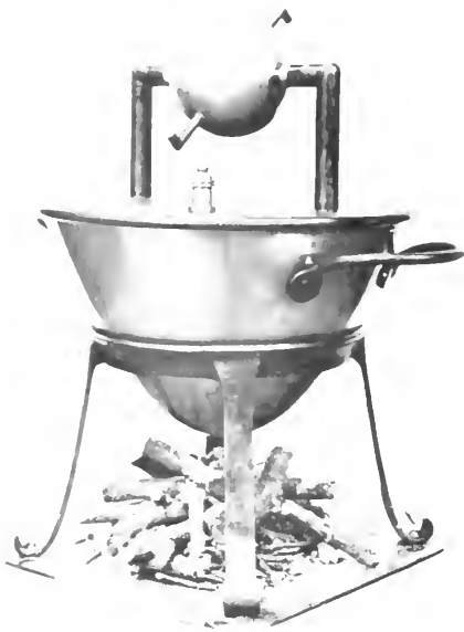
A model of Heron's aeolipile. Steam produced in the boiler escapes through the nozzles on the sphere, causing the sphere to rotate.
