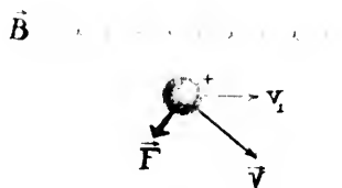
(c) If \vec{v} is not perpendicular ( \perp ) to \vec{B} , there is a smaller force, proportional to v_{\perp} instead of v .
