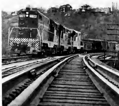
An engine starting abruptly can start a displacement wave along a line of cars.
