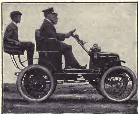
FIG. 117.—“ Automotor ” Gasoline Phaeton, with rumble seat, illustrating a recent design in light motor carriage construction.
