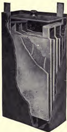
FIG. 375.—One Cell of the "Gould" Storage Battery for Electric Vehicle Use. According to the data given by the manufacturers, this cell, containing four negatives and three positive plates, has a normal charging rate of 27 amperes; a distance rate of 22\frac{1}{2} amperes for 4 hours; a capacity of 81 ampere-hours at 3 hours' discharge, and of 90 ampere-hours at 4 hours' discharge. The plates are each 5\frac{7}{8} \times 7\frac{3}{4} inches, and the total dimensions of the cell, enclosed in its rubber jar, are 2\frac{1}{2} \times 6\frac{1}{4} \times 11 inches. Forty such cells are generally used for an average light vehicle battery.
