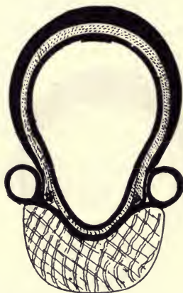
FIG. 102.—The Dunlop Double-Tube Tire. The attachment is at the base of the inner tube by the endless wires shown, which are pressed against the tubular sides of the rim channel when the tire is inflated, thus affording a positively immovable hold.
