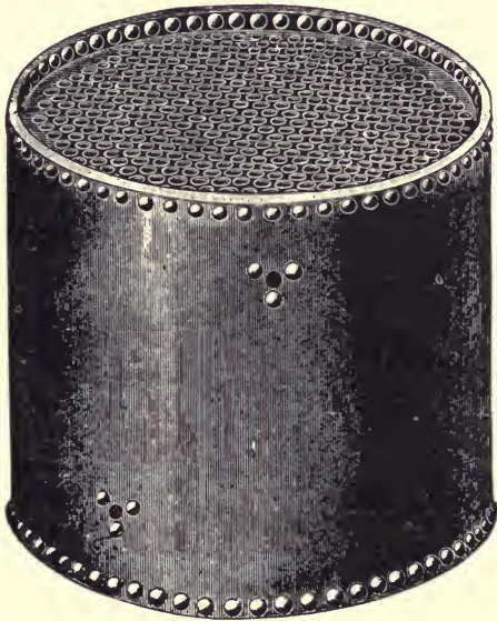
FIG. 403. —Another type of Small Carriage Boiler, showing both tube plates inlanged and riveted to a seamless steel tube.
