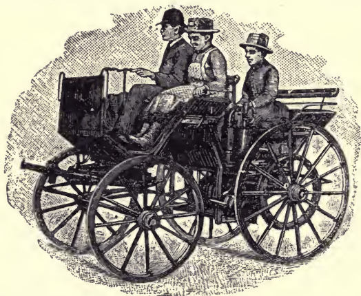
FIG. 260.—The First Daimler Motor Carriage. The motor was connected to the driving axle by two belts; one for high speed, the other for climbing; either being thrown into action as the belts were tightened by jockey pulleys, as shown in Fig. 261. Both could be thrown out of action to stop the carriage without stopping the motor. The forward axle of this carriage was centre-pivoted and turned on a fifth wheel, as in horse carriages; the steering being by upright pillar rising before the driver's seat.
