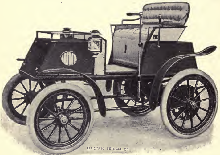
FIG. 336. —“Columbia” Electric Runabout. This carriage, weighing about 1,900 pounds, has a traveling radius of about forty miles per full charge of battery, and a maximum speed of thirteen miles per hour.
