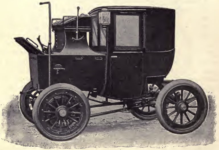
FIG. 59.—Front-Driving Brougham of the Electric Vehicle Co., used in New York City. This model, which is no longer manufactured, represents a construction very suitable for city service, but quite inappropriate for country and general use.
