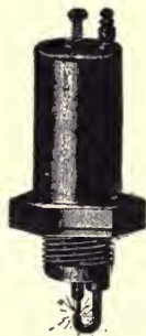
FIG. 189.—Details of a Common Form of Contact for Producing a Wiping Spark. The electrode, X , rotated by the crank, E , as indicated, gives a wiping contact and break at the terminal, Y , which is tipped by a resilient platinum spring. One of the wires forming the circuit is connected at D through the insulated plug screwed into the body of the ignition chamber; the other is connected to the metal of the chamber at the nut, M . The advantage of this form of sparking device is that the constant contact of the electrode keeps the surfaces clean, but at the same time the constant friction produces an immense wear for the same reason. An excellent form of simple make-and-break device is shown in connection with the suction of the Duryea cylinder in a succeeding chapter.
