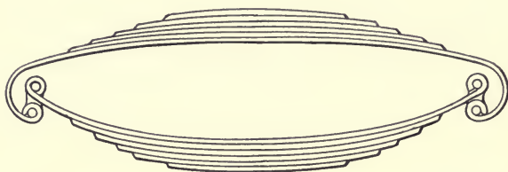
FIG. 82.—Rear Spring used on the Packard Light Car. The C-shaped upper portion is connected by shackles to the elliptical lower half, the effect being to allow the use of fixed distance rods and keep the chain taut, without the use of the usual devices of foreign and American carriages.
