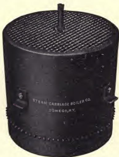
FIG. 401.—Small Carriage Boiler made from a seamless steel pressing, the lower tube plate being flanged over and riveted in, as indicated at the base of the figure, this being the only seam in the structure.
