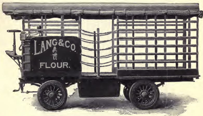
FIG. 340.—Heavy truck of the Vehicle Equipment Co. Carrying capacity, 4 tons; speed, 6 miles per hour; travel radius on one charge of battery, 25 miles.
