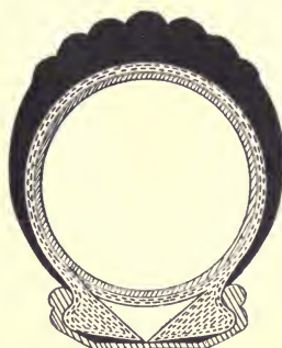
FIG. 101.—The G. & J. Tire. Like the Michelin Tire, this is attached at the base by the fit of the case tube and rim channel, being securely held when the tire is inflated. A flap on the case tube saves the inner tube from pinching at the base.
