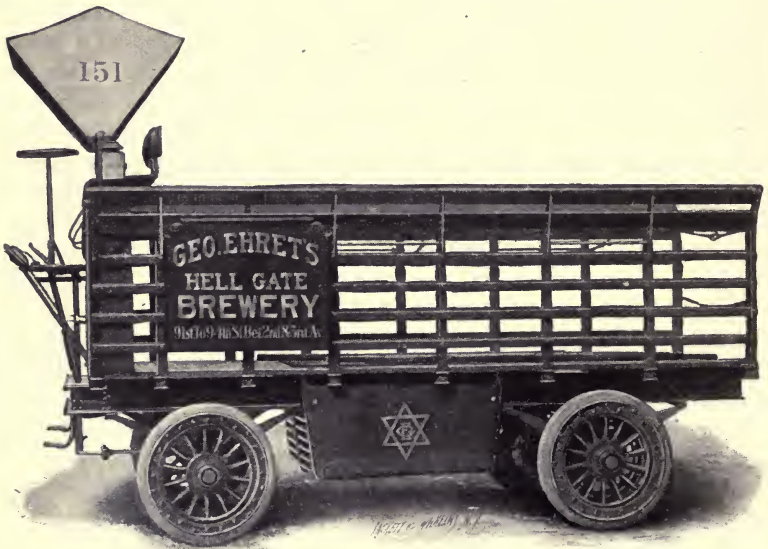
FIG. 357.—Electric Brewery Wagon of the Vehicle Equipment Co. Carrying capacity, 5 tons; speed, 6 miles per hour at full load; travel radius on one charge, 25 miles.
