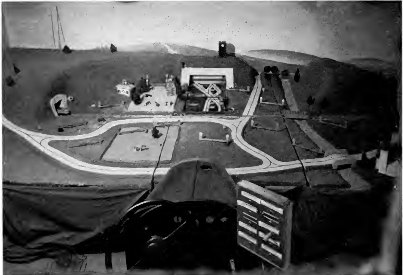
Fig. 1. The Drivometer. This device for simulating driving has been used at Iowa State University for a number of years. Several studies and masters' theses and a doctor's thesis have been done using this as the basic apparatus. A regular car seat is mounted in the mockup car body in the foreground. From numerous studies it is estimated that about 25% of the variance (factors involved in driving) is measured.
