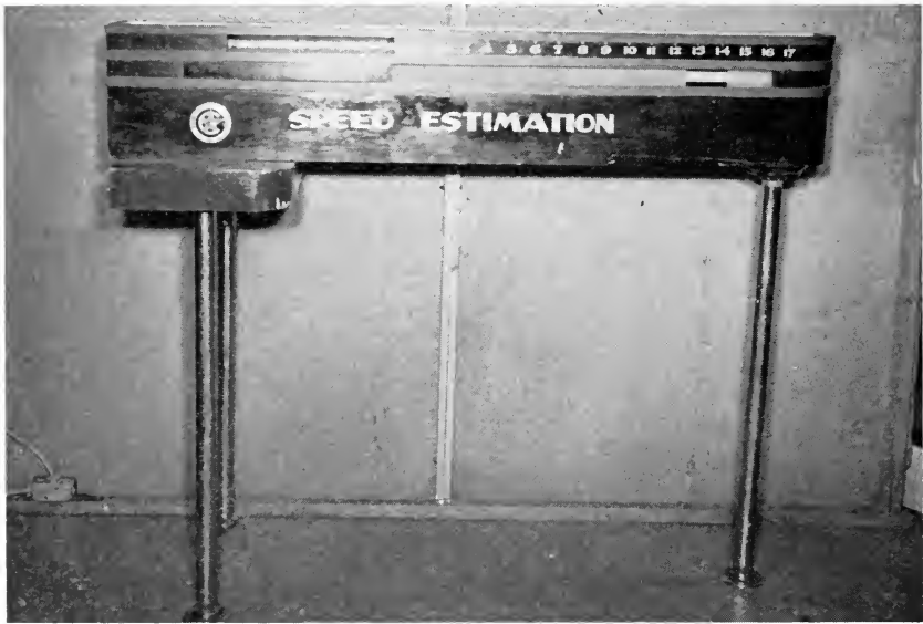
Fig. 7. Speed Estimation. In this apparatus, a small car travels across the opening and behind the numbers. The panel shown just below the numbers is lighted; when the car passes a preselected number, the light goes off. The subject is to judge the position of the car at that instant. (Courtesy, Chicago Motor Club.)
