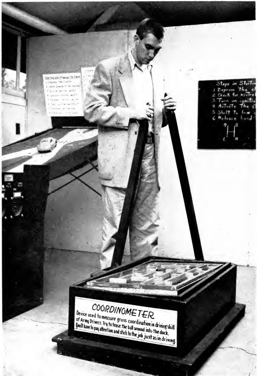
Fig. 6. Coordinometer. Gross coordination was used to classify Army driving personnel and was found to be one of the most effective.
