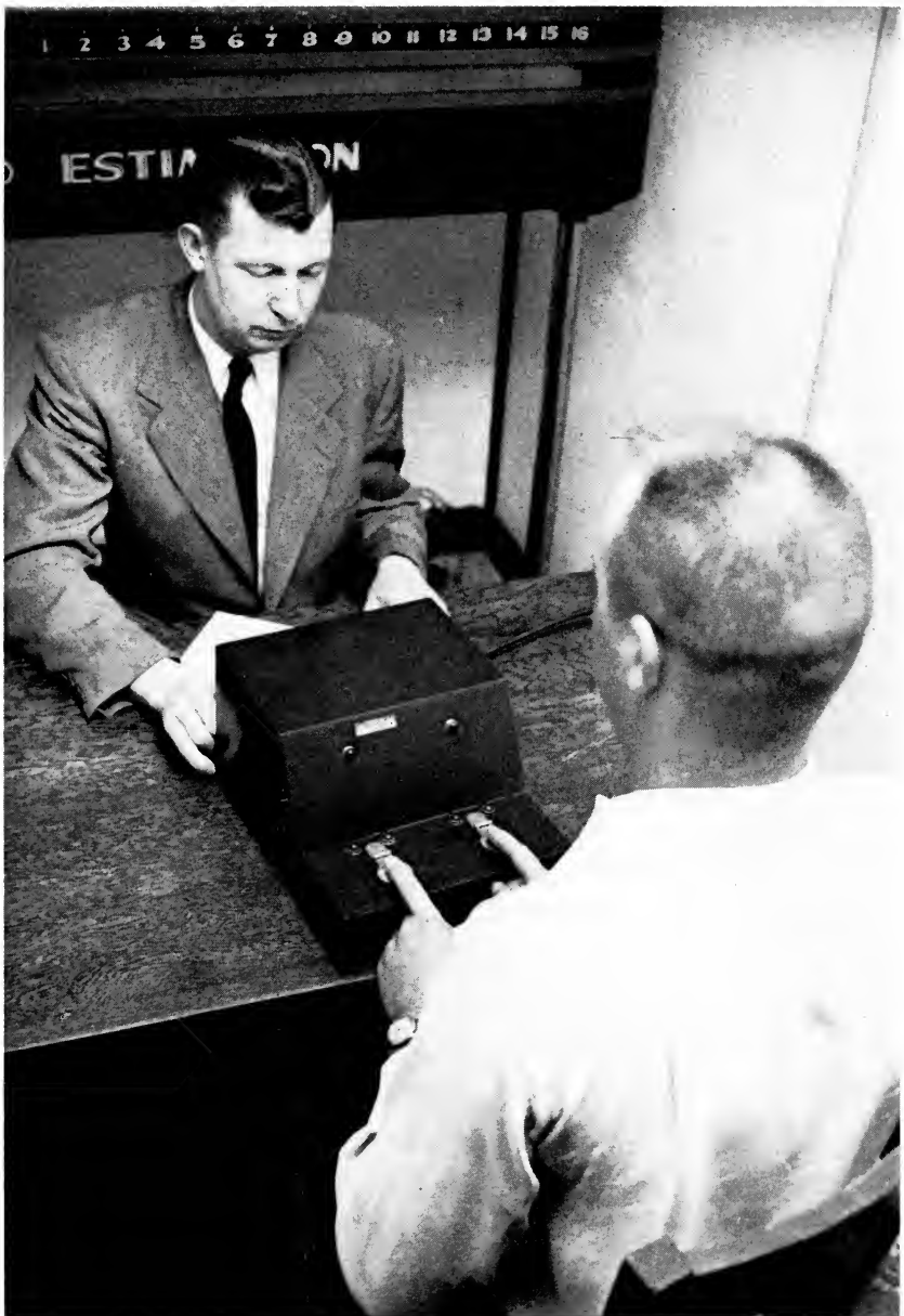
Fig. 8. Choice Reaction Time. The subject reacts to each of the light combinations given by the experimenter. The time clock is at the back for ease of reading.
