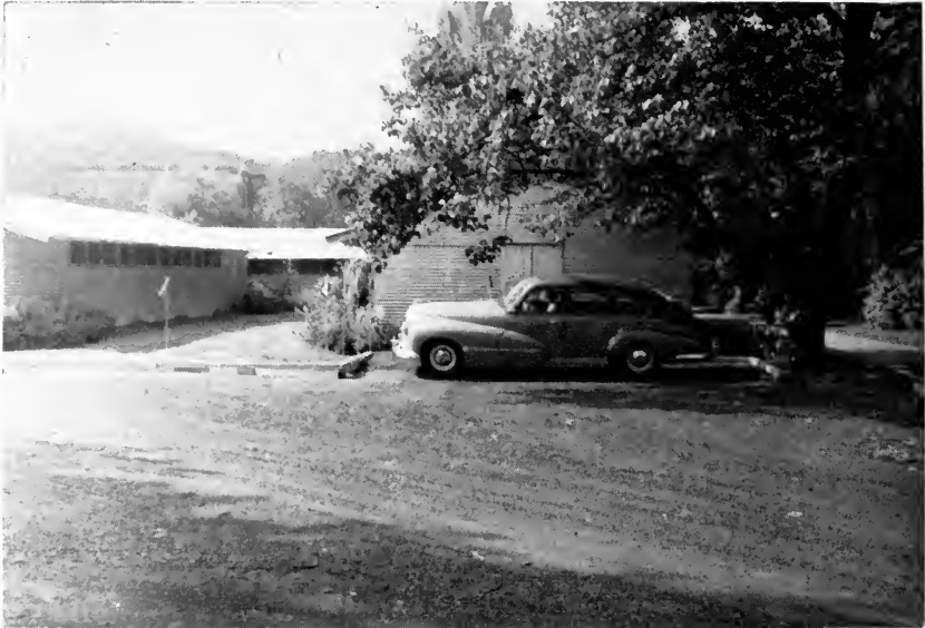
Fig. 2. Parallel Parking Stall. Ordinarily 5 feet over the length of the car is needed for satisfactory parking. An ordinary driver should park correctly in 50 to 70 seconds and make no extra hitches or moves. One operator, properly trained, could handle from three to five of these stalls at once, thus speeding up the examination of drivers.
