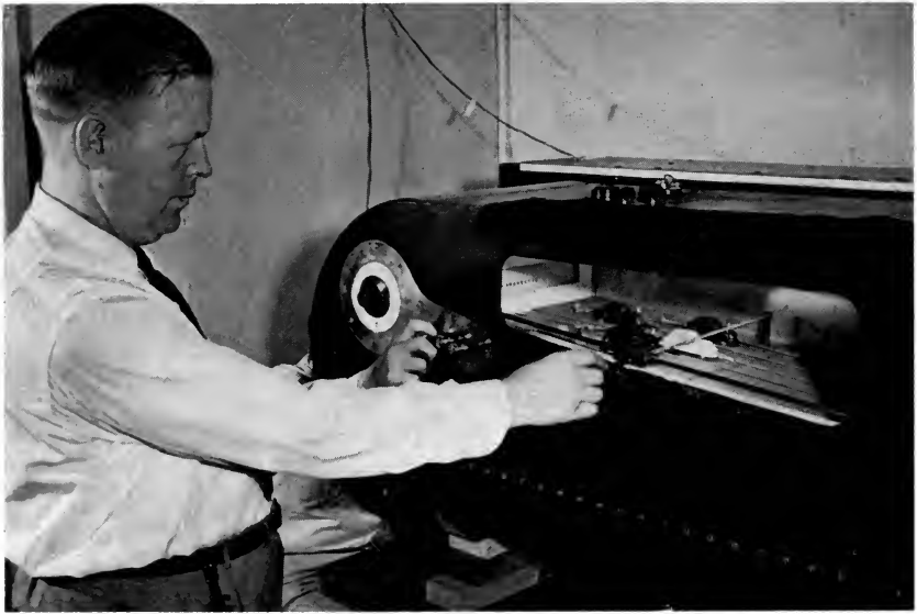
Fig. 4. Distance Judgment. One form of distance judgment apparatus is shown. The subject sees the cars in the mirror at about 8 feet effective distance. He looks into the end and sets the cars with the round knobs.
