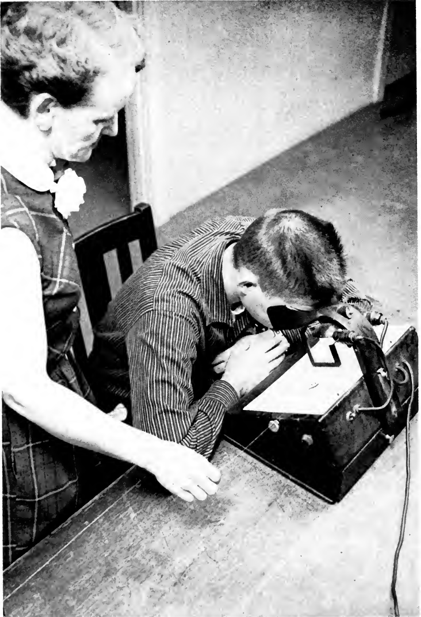
Fig. 13. The Cheiroscope. This apparatus is used to diagnose defects of vision such as scotoma and use of the eyes together. It may also be used to determine blind spots in the visual field.
