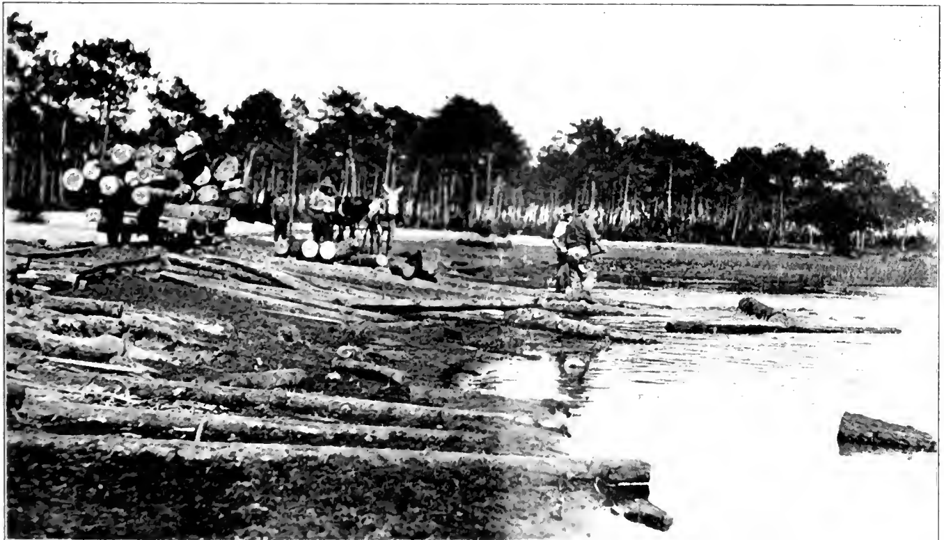
CAR LOAD OF MARITIME PINE LOGS BEING DUMPED INTO AUREILHAN LAKE TO BE TOWED TO THE AUREILHAN AMERICAN SAWMILL NEAR PONTENX, LANDES. NARROW GAUGE RAILWAY SHOWN. THE MULES BRING THE LOGS FROM THE PINE FORESTS OF THE SAND DUNES.
