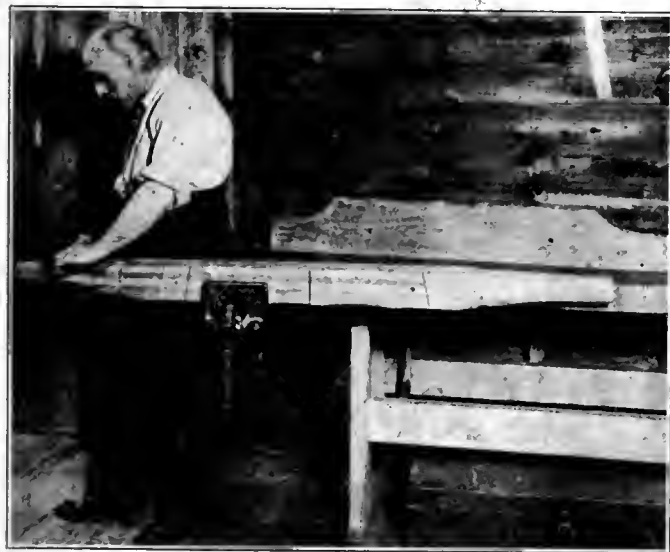
BUT LITTLE IS KNOWN AT PRESENT CONCERNING THE EFFICIENCY OF BUILT-UP AXLES AND BOLSTERS SUCH AS THOSE SHOWN IN THE ILLUSTRATION. THEY WOULD UNDOUBTEDLY BE STRONG ENOUGH TO DO THE WORK EXPECTED OF THEM, BUT NO DATA IS AS YET AVAILABLE TO SHOW HOW MUCH RESISTANCE THEY WOULD HAVE AGAINST EXPOSURE TO THE WEATHER AND THE SHOCKS INCIDENT TO USE.
