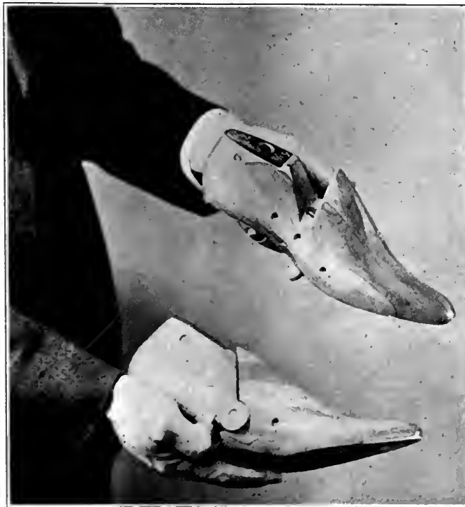
TWO TYPES OF LAMINATED SHOE LASTS ARE ILLUSTRATED IN THIS PHOTOGRAPH. THE UPPER LAST IS MADE WITH VERTICAL LAMINATIONS AND THE LOWER ONE WITH HORIZONTAL LAMINATIONS. THESE LASTS ARE USED IN THE MANUFACTURE OF SHOES AND RECEIVE A MUCH HARDER SERVICE THAN THE ORDINARY SHOE TREE. THE SOLID LASTS ARE USUALLY MADE OF MAPLE AND BIRCH AND THE LOSSES INCURRED IN THE SEASONING OF THE BLOCKS AND THE MANUFACTURE OF THE LASTS ARE NORMALLY RATHER GREAT. SEVERAL SHOE FACTORIES ARE COOPERATING WITH THE FOREST PRODUCTS LABORATORY IN TESTING OUT THE SERVICEABILITY OF THE LAMINATED LASTS. WHILE NO DEFINITE RESULTS HAVE AS YET BEEN OBTAINED, PRESENT INDICATIONS ARE THAT LAMINATED LASTS, BUILT UP WITH WATER-RESISTANT GLUES WILL BE QUITE SATISFACTORY.
