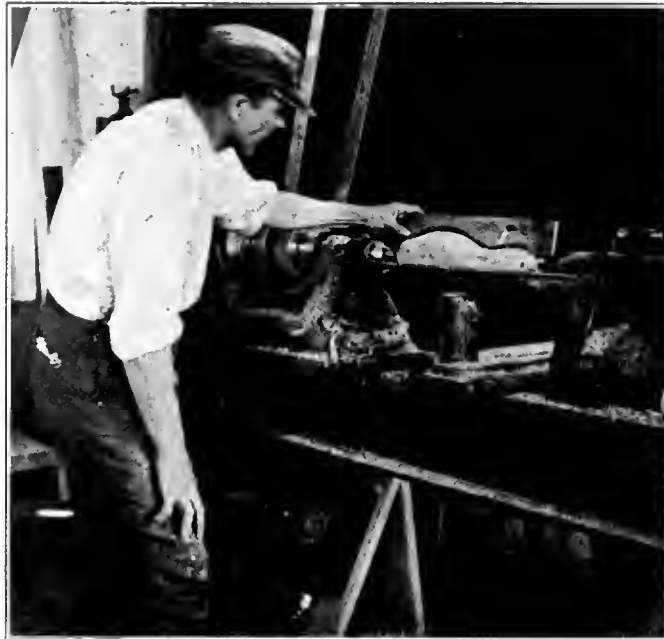
IN THE MANUFACTURE OF LAMINATED BOWLING PINS THE BLOCK HAVING BEEN ROUGHED OUT ON THE BAND SAW IS PUT IN THE TURNING LATHE AND TURNED TO THE PROPER PATTERN. AFTER A SUITABLE FINISH HAS BEEN APPLIED THE PINS ARE READY FOR TEST.
