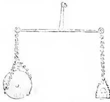
Fig. 4473. — Balance à contrepoids.
