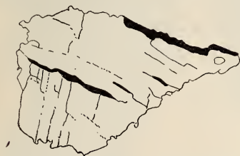
FIG. 4.—Natural Widmanstätten figures brought out by burnishing.
