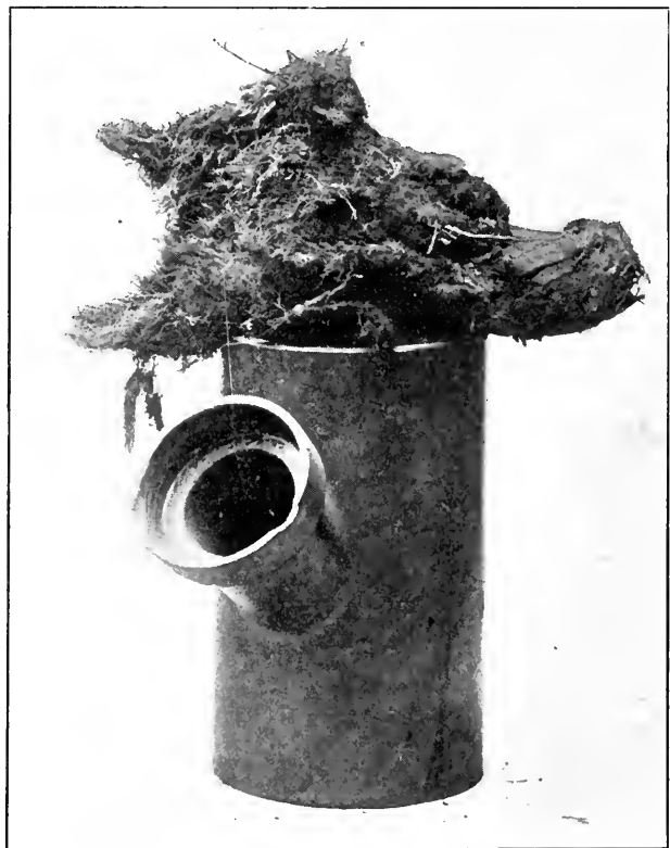
ELM ROOT FROM SEWER PIPE.
