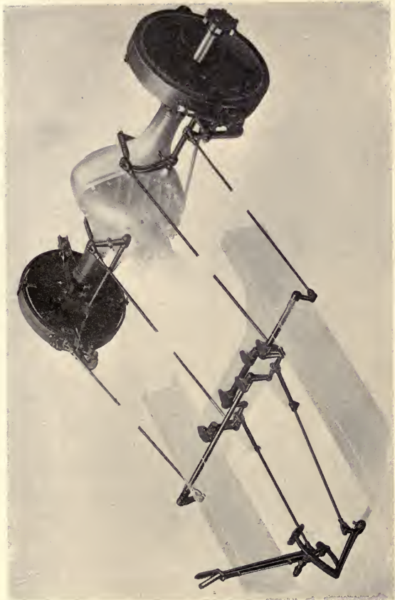
4 BRAKE LEVERS AND LINKAGE, SHOWING EQUALIZING ROD AND SPRINGS
