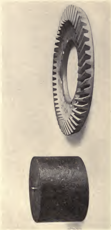
CYLINDER OF STEEL, AND THE GEAR WHEEL WHICH WAS HAMMERED FROM IT
