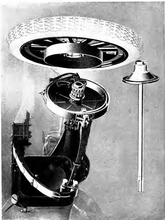
REAR WHEEL AND BRAKE DRUM REMOVED, SHOWING EXTERNAL AND INTERNAL BRAKE BANDS AND MECHANISM
