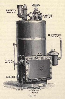
These coils being the hottest part of the apparatus, the mineral deposits thrown down by the boiling sea-water tend to adhere to them; but from the constantly varying temperature outside and inside the coils, they expand and
