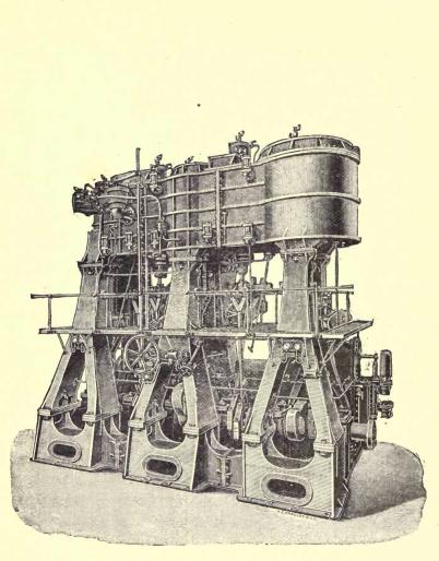
TRIPLE EXPANSION ENGINES OF P. & O. S.S. "ADEN."
