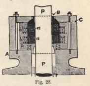
(C), which is bolted on to the cylinder cover. It has been found that the wear on the composition blocks (*aa*), Fig. 28, was only  $\frac{3}{64}$  of an inch, after the engines to which this packing was fitted had run 24,000 miles, and there are many cases in which the packing had been run 150,000 miles without repairs.
