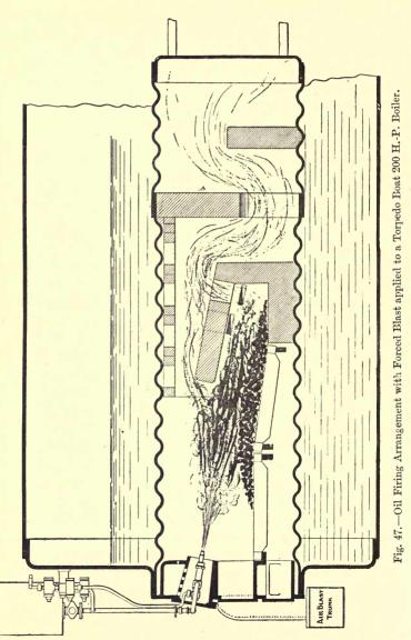
only to equalise the rate of steam production, but prevents the passage of the unburnt or unoxidised hydrocarbons into the tubes of the boiler.
