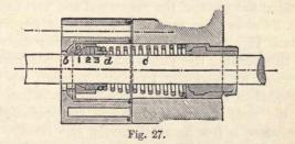
and 3, each having a small portion cut out to allow them to tightly clasp the rod; these three rings fit into a vibrating cup (a), which presses against a ball-andsocket-joint (b); this joint and the one between the
