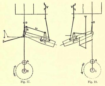
The advantages of this gear are that, by dispensing with eccentrics, the engine is somewhat shortened in the ship, and access to the main bearings and connecting rods is much facilitated. It is only applicable where the valves are at the back of the cylinders.
