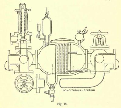
There is also a by-pass pipe uniting the two branches of the feed-pipe, thus the feed can pass through either or both filters, or through the by-pass pipe to the boiler. To use the language of electrical engineers, the filters and the by-pass are in "parallel arc," and are
