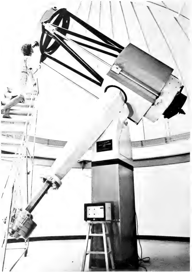
Fig. 1. Observer at the Newtonian focus of the 30-inch reflector. The photographic equipment (camera, offset guiding microscope, and small finder) can be mounted at any of four observing stations spaced around the ring beam at the top of the tube.
