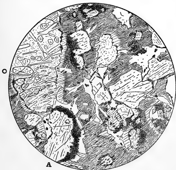
Fig. 1.— Hornblende-peridotite from Glendalough, showing pœcilitic structure in hornblende (shaded) with tremolite-rims (unshaded).
