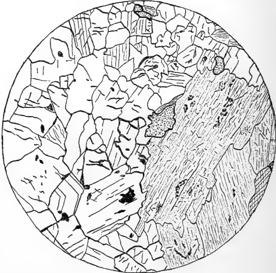
Fig. 5.— Clinozoisite-vein in amphibolite from Glendalough, showing clinozoisite, hornblende, and sphene. (Magnified 30 diameters.)
