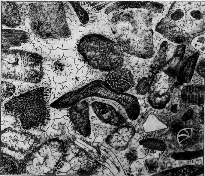
Fig. 2.—CORALLINE OOLITE, SCARBOROUGH, \times 50 DIAMS.
