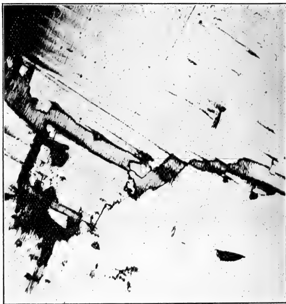
Fig. 11.— Strings of native silver in galena: Foxdale Mine, Isle of Man. (Reflected light: \times 400 .)
