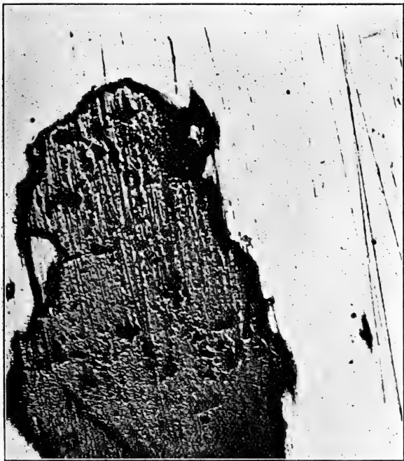
Fig. 9.— Blende, with rough-pitted surface, enclosed in galena: Halkyn Mine, Flintshire. (Reflected light: \times 200 .)
