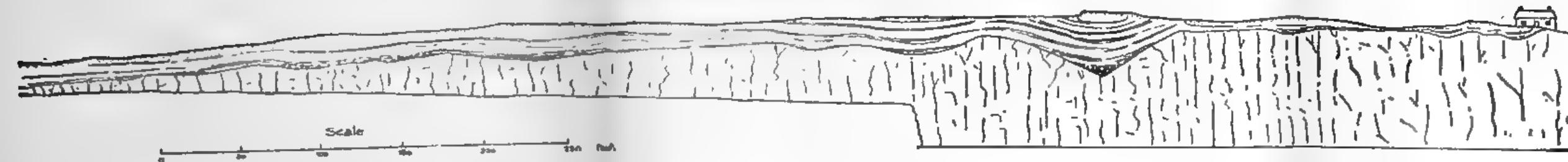
Fig. 2.—Section at Sheet Hedges Wood Quarry, Groby, showing catenary bedding in a gully.
